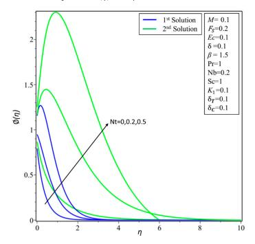
**Figure 15.** Variation of nanoparticle volume fraction  $\varphi(\eta)$  with  $\eta$  for several values of thermophoresis parameter  $N_t$ .
