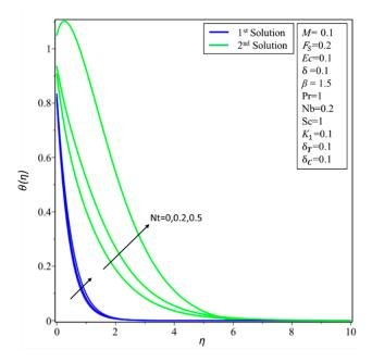
**Figure 12.** Variation of temperature  $\theta(\eta)$  with  $\eta$  for several values of thermophoresis parameter  $N_t$ .
