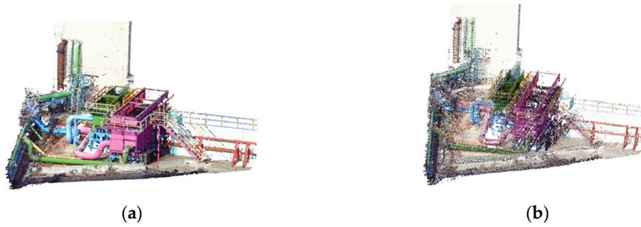
**Figure 5.** (a) Prebuilt point cloud data set and (b) optimal subsampled point cloud.
