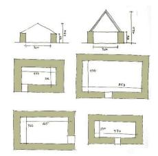
**Figure 18.** Cross-sections through two types of gladas and examples of plans of gladas of different dimensions, drawing: A. Kapetanović.
