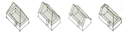
**Figure 13.** Variants of gladas' walls: a leveled sidewall, one gable wall, two gable walls and a half-gable wall drawing: A. Kapetanović.
