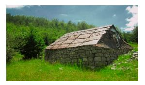
**Figure 16.** Glada with its face oriented parallel to the terrain, partially dug into the ground—Građen, Podgradski katun, photo: I. Laković.
