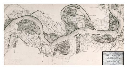
**Figure 2.** Po River. Table X, called Mortizza (Piacenza province). Map of the River Po, from Ticino to the sea (from direct surveys carried out in 1821 and updated in 1853), at a scale of 1:15,000 by Corpo Reale del Genio Civile. Archive CNR IRPI Turin.
