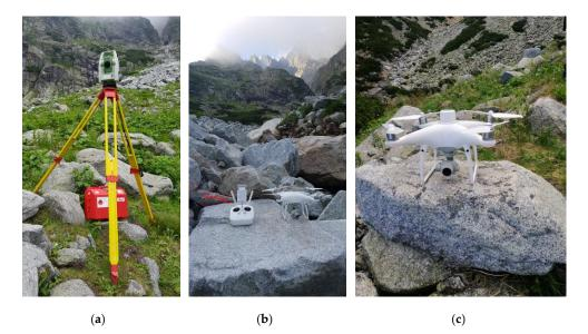
**Figure 3.** Instruments and equipment. (**a**) Leica TS02 total station, (**b**) DJI Phantom 4 UAS, (**c**) DJI Phantom 4 RTK UAS.
