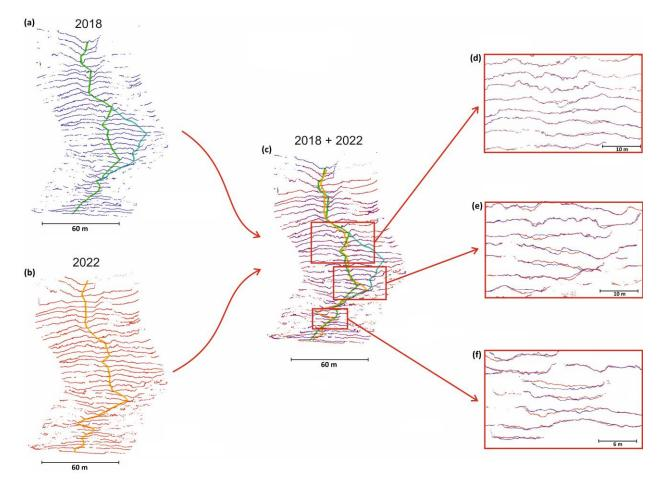
**Figure 11.** DTM display of talus cone cross-sections (10 m spacing). (a) 2018 data, (b) 2022 data (c) 2018 and 2022 data combined. Bed of the tidal stream shown by green, blue-green, and orange lines. (**d**–**f**) Three details where significant changes are visible.
