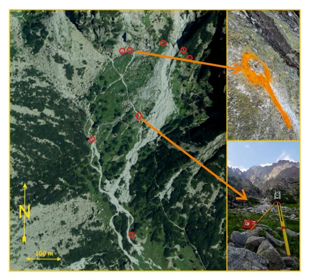
**Figure 2.** Geodetic network points. Circles mark the points of the geodetic network, rhombus indicates the position of the total station. Map source—maps.google.com, accessed on 12 January 2023.
