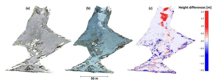
Figure 8. Horizontal view in the direction of the talus cone. (a) 2018 data, (b) 2022 data, (c) color-coded height differences in the 2022 cloud.
