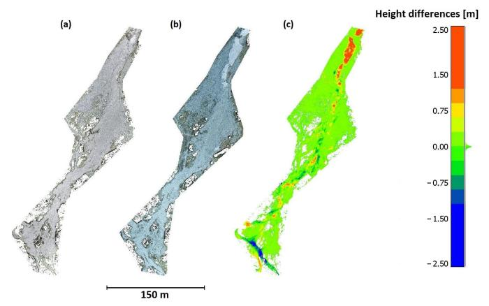
Figure 9. Top view. (a) 2018 data, (b) 2022 data, (c) color-coded height differences in the 2022 cloud.
