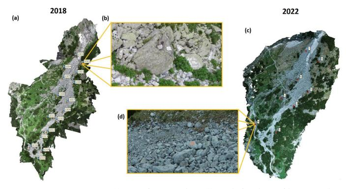
**Figure 4.** (a) Position of GCPs in epoch 2018, (b) example of signalization of the GCP in epoch 2018. (c) Position of GCPs in epoch 2022, (d) example of signalization of the GCP in epoch 2022.
