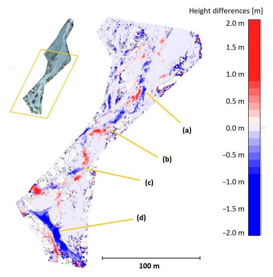
Figure 12. Details of the lower part of the monitored area with visible changes marked by (a-d).
