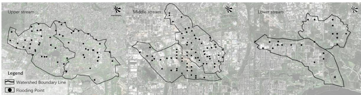
**Figure 4.** The distribution of overflow nodes with overflows exceeding  $10 \times 10^4 \text{ m}^3$ .
