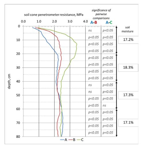
**Figure 11.** Soil cone penetrometer resistance measured in October 2021 (A—no traffic; B—single pass; C—multiple passes/permanent tramlines) and comparison of differences between the areas (one way ANOVA,  $\alpha = 0.05$ ; ns = not significant).
