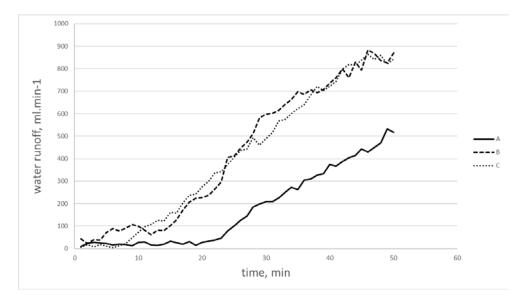
**Figure 9.** Intensity of water runoff measured in three locations during the simulated rain with the intensity of 1300 mL min<sup>-1</sup>: (A) no traffic area; (B) single pass area; (C) multiple pass/permanent tramline area.
