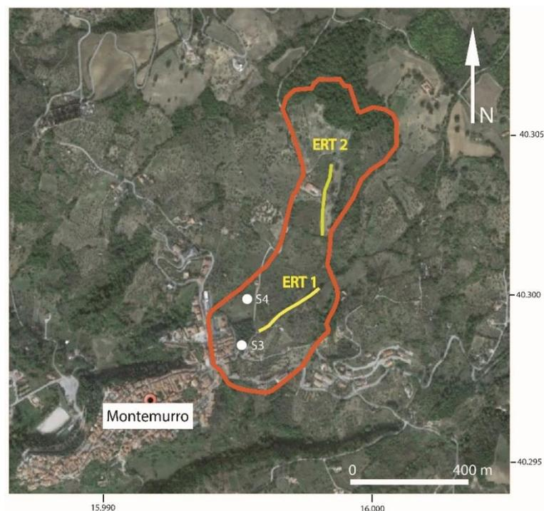
**Figure 9.** Traces of the two ERT (in yellow) and the limit of the Servigliano landslide (in orange). Satellite image from Google Earth™. The map also shows the two boreholes (S3 and S4).
