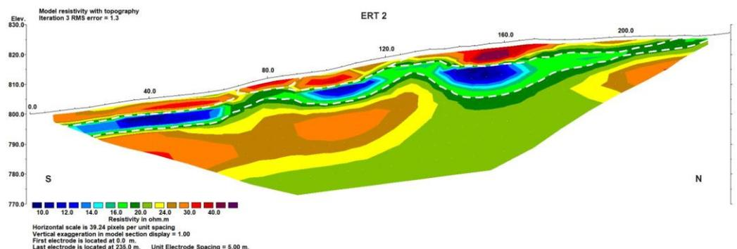
**Figure 11.** Electrical resistivity tomography (ERT 2) carried out parallel to the landslide body along the middle part. Dashed white lines outline possible sliding surfaces. Elev.: elevation above sea level.
