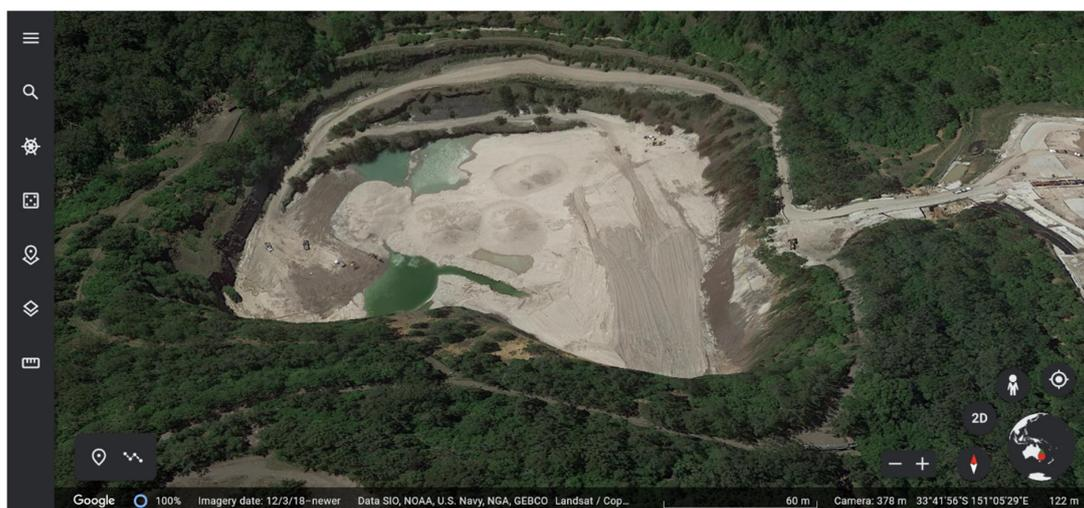
**Figure 5.** Current aerial view of the Hornsby Quarry, facing north (Google Earth image, dated 12 March 2018), showing partial infilling of the quarry by spoil. Scale bar shown is 60 m.
