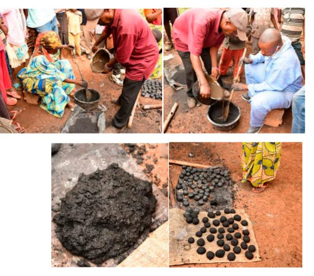
**Figure 5.** Steps in making briquettes by smallholder farmers supported by a local non-governmental organization, DIOBASS, in eastern DRC.
