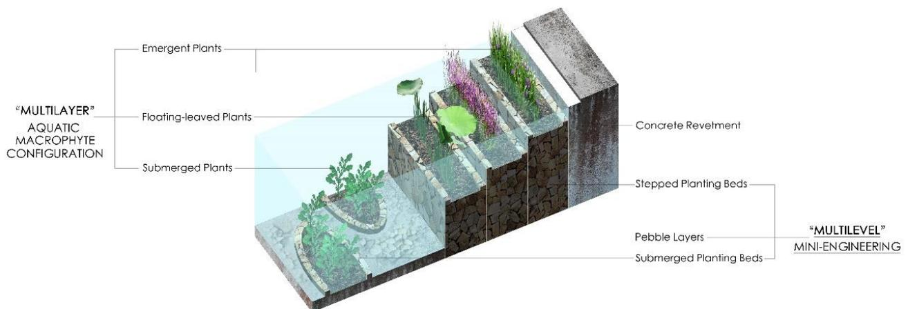
**Figure 9.** Sectional perspective of the in situ ecological self-purification model.
