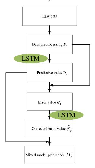
Figure 8. LSTM-SVR hybrid model framework diagram.
