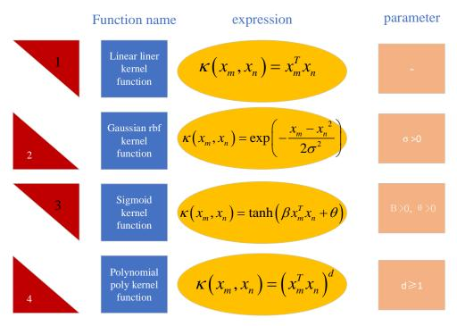
Figure 7. Schematic diagram of kernel function names and characteristic parameters.
