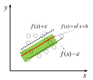
Figure 6. Schematic diagram of SVR.
