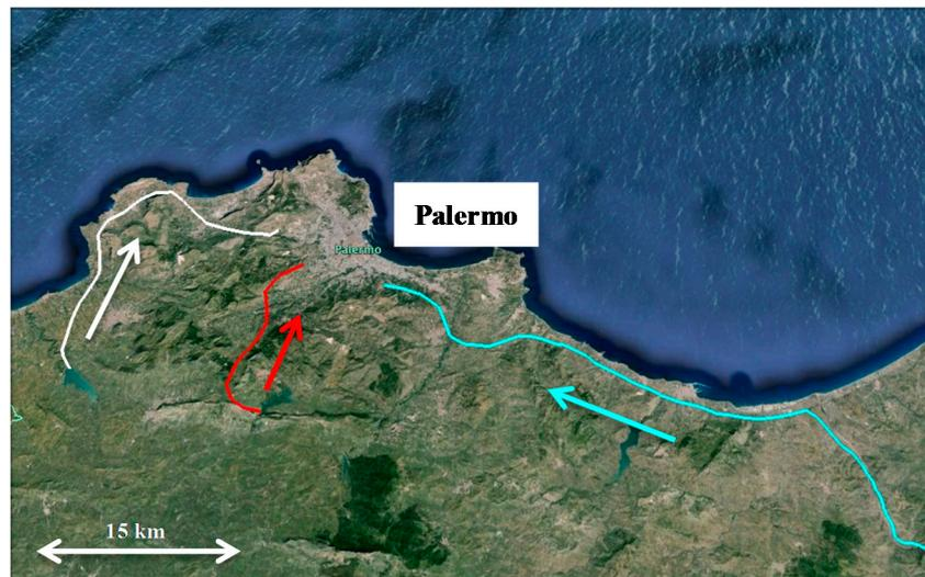
**Figure 2.** Water supply scheme in Palermo: Jato system (white); Gabriele System (red) and Scillato System (cyan).
