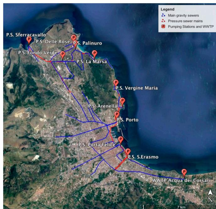
Figure 5. Diagram of the main sewer system and pumping station.
