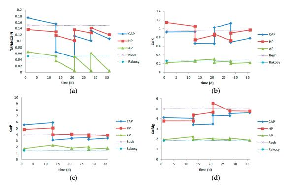
**Figure 1.** LS mean of macronutrient concentration ratio evolution in complemented aquaponic (CAP), hydroponic (HP), and aquaponic (AP) treatments during trial 2. Resh's and Rakocy's ratios are given for comparison. (a) TAN to  $NO_3^-$ -N ratio; (b)  $Ca^{2+}$  to  $K^+$  ratio; (c)  $Ca^{2+}$  to P ratio; (d)  $Ca^{2+}$  to  $Mg^{2+}$  ratio.
