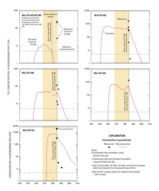
**Figure 3.** Reconstructed (simulated) and measured concentrations of trichloroethylene (TCE) at selected water-supply wells within the Hadnot Point Industrial Area and the Hadnot Point landfill area at U.S. Marine Corps Base Camp Lejeune, North Carolina (modified from [1]).
