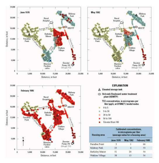
**Figure 5.** Reconstructed (simulated) distribution of trichloroethylene (TCE) contamination within the Holcomb Boulevard water treatment plant service area resulting from supply of contaminated Hadnot Point drinking water, June 1978, May 1982, and February 1985 (from [1,12]; 1 ft = 0.3048 m).
