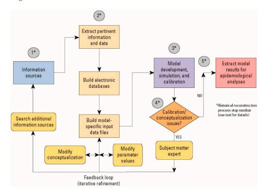
**Figure 2.** Generalized process of identifying information, extracting usable model-specific data, and applying models to reconstruct historical drinking-water contaminant-specific concentrations (from [1]).
