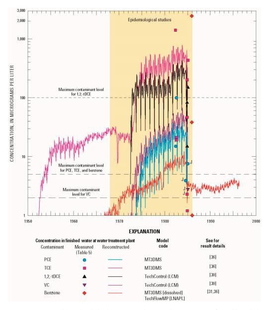
**Figure 4.** Reconstructed (simulated) drinking-water and measured concentrations of tetrachloroethylene (PCE), trichloroethylene (TCE), *trans*-1,2-dichloroethylene (1,2-tDCE), vinyl chloride (VC), and benzene at the Hadnot Point water treatment plant, U.S. Marine Corps Base Camp Lejeune, North Carolina. (See [1] for a listing of monthly mean drinking-water concentrations; J, estimated; LCM, linear control model; LNAPL, light nonaqueous phase liquid.)
