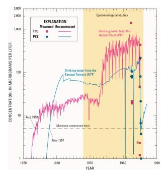
**Figure 6.** Reconstructed (simulated) drinking-water and measured concentrations of tetrachloroethylene (PCE) and trichloroethylene (TCE) at the Tarawa Terrace and Hadnot Point water treatment plants, U.S. Marine Corps Base Camp Lejeune, North Carolina (from [1,4,5]).
