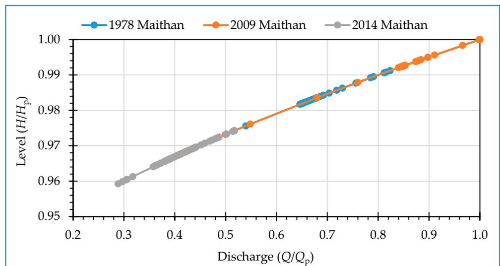
**Figure 5.** Non-dimensional variation in reservoir discharge with elevation of Maithan Dam.
