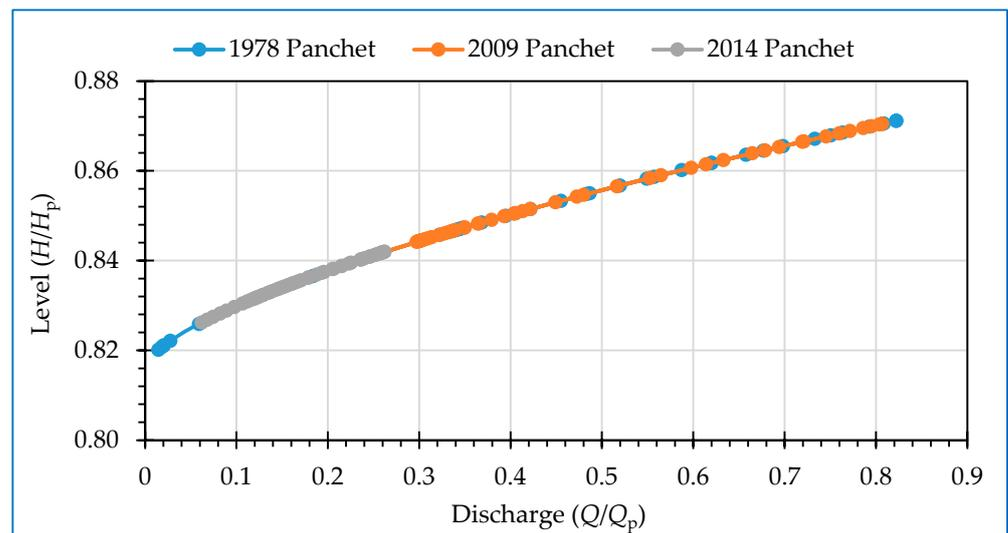
**Figure 6.** Non-dimensional variation in reservoir discharge with elevation of Panchet Dam.
