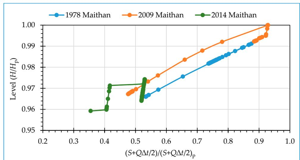
**Figure 3.** Non-dimensional variation in reservoir storage with elevation or level of Maithan Dam.
