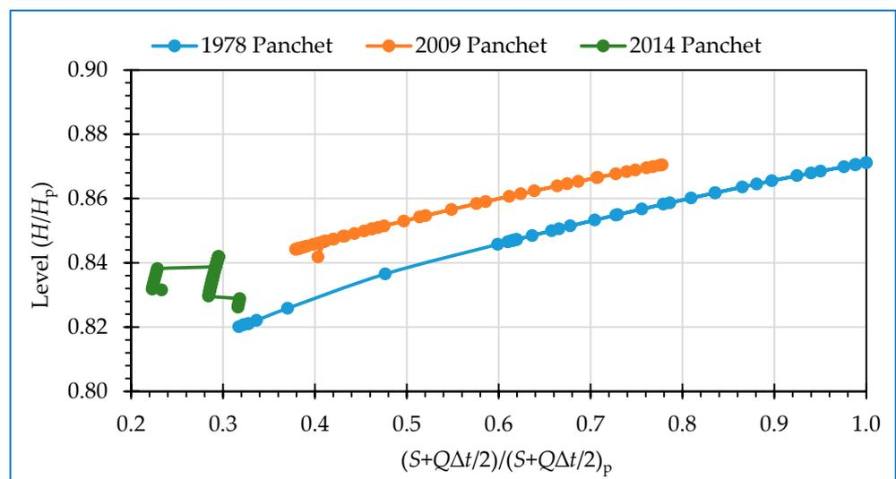
**Figure 4.** Non-dimensional variation in reservoir storage with elevation or level of Panchet Dam.
