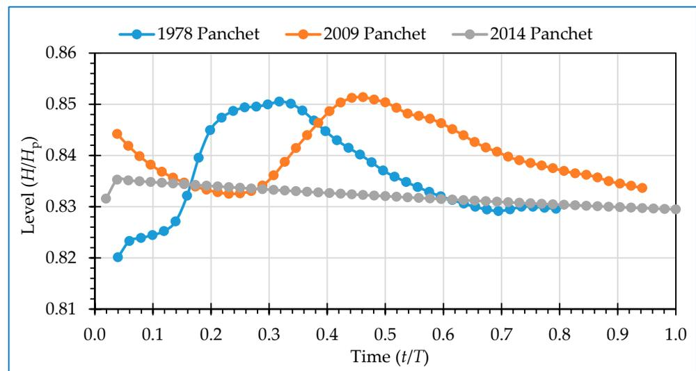
**Figure 8.** Non-dimensional variation in reservoir elevation with time of Panchet Dam.
