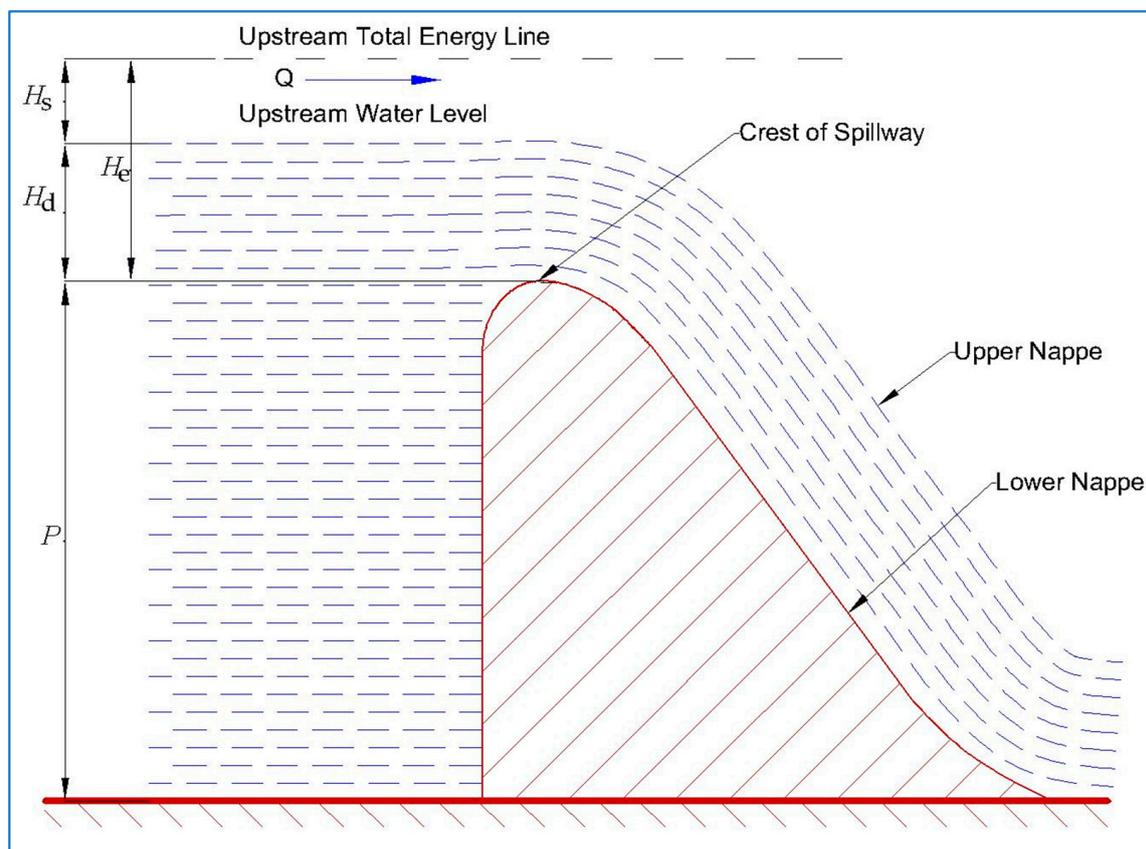
Figure 2. Profile of a gated ogee spillway.
