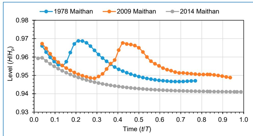
**Figure 7.** Non-dimensional variation in reservoir elevation with time of Maithan Dam.
