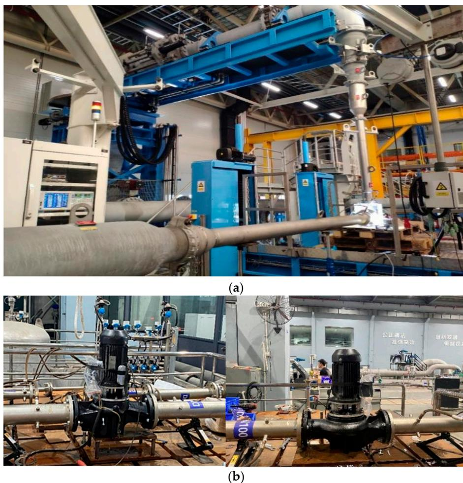
**Figure 8.** Closed test bench construction of the original pump visual model. (a) A closed test platform for comprehensive testing of pump performance; (b) a prototype pump visual model.
