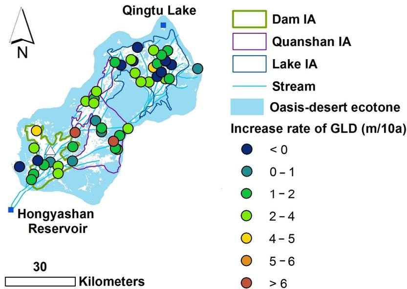
Figure 9. Change rate of the groundwater depth during 2009–2017.
