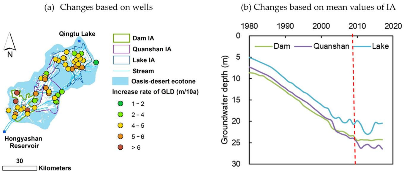
**Figure 3.** Changes in the groundwater depth in the irrigation areas of Minqin Oasis during 1980–2017 (GLD: groundwater depth; IA: irrigation area; the red dotted line represented the turning point year).
