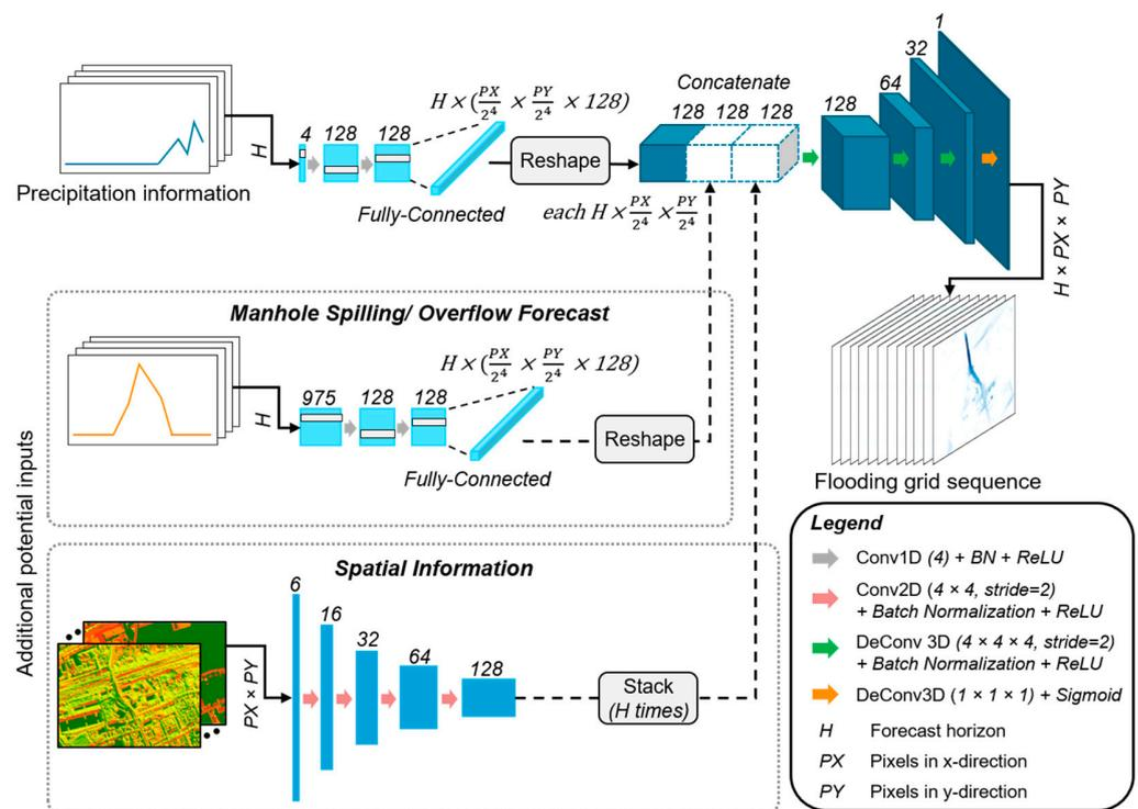
**Figure 6.** Baseline architecture combined with the corresponding input paths for the overflow forecast and the spatial information.
