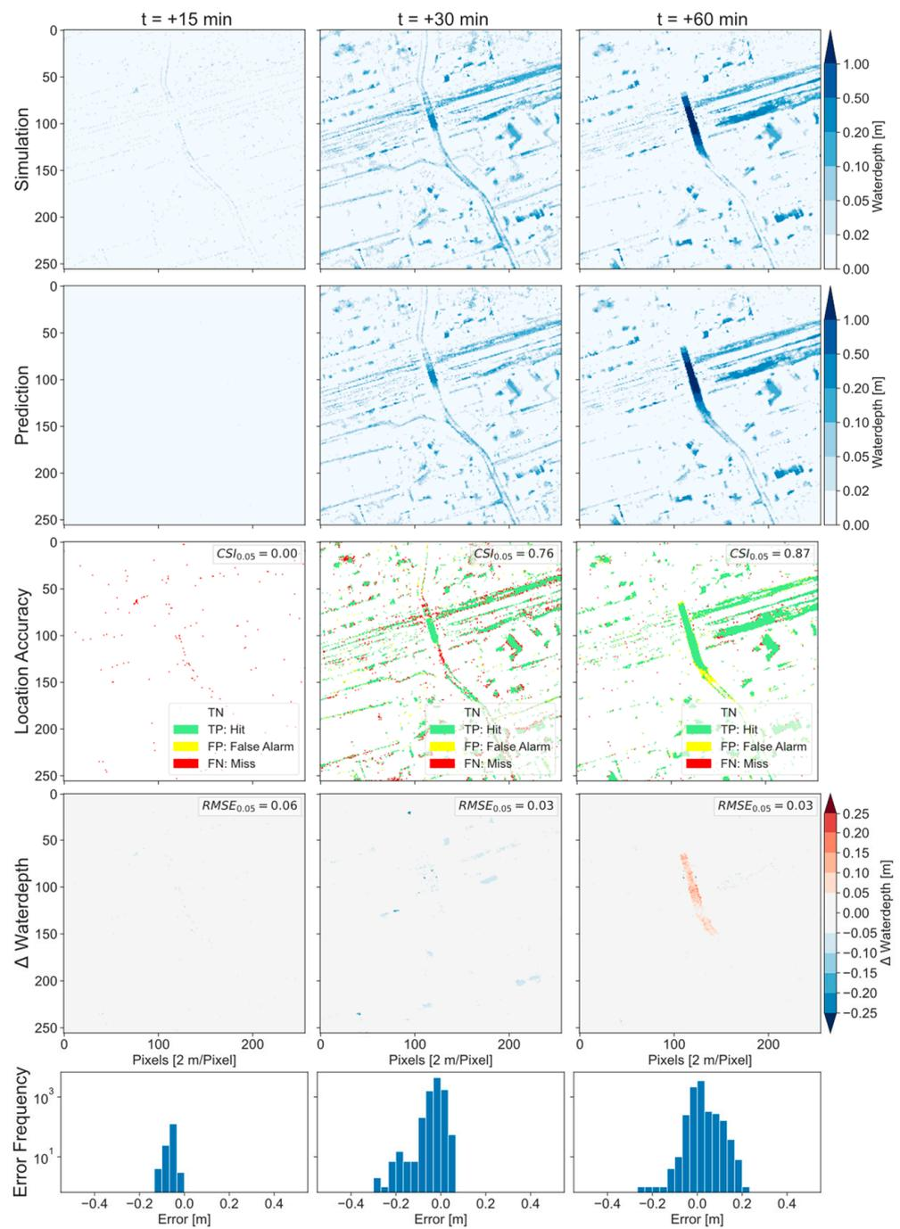
**Figure 13.** Results and evaluation for three time steps of a single forecast with the T-GCN at the beginning of the event on 3 July 2009 in Gelsenkirchen. Instead of showing the entire study area, a section with a flooded underpass is expanded for better visualization.
