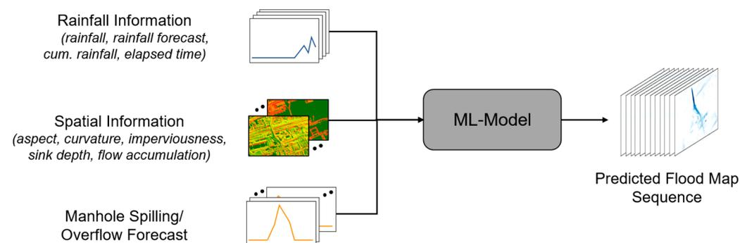
**Figure 1.** Model setup with all potential inputs (**left**) and the target variable (**right**).
