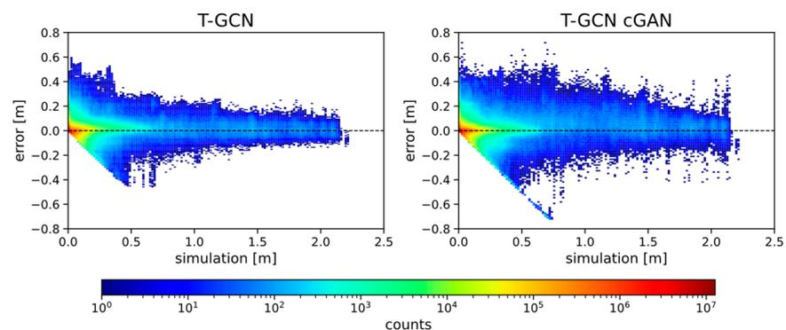
Figure 12. The 2D histogram with the prediction error as a function of the simulated water depths.
