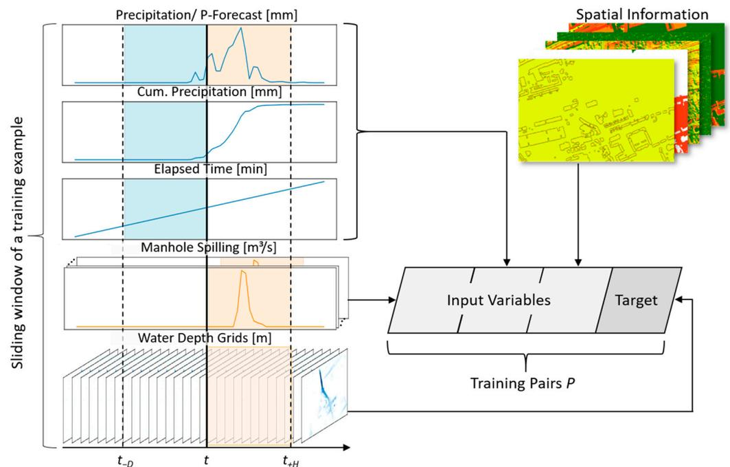
**Figure 4.** Converting the data into a supervised learning problem using a single training pair as an example.
