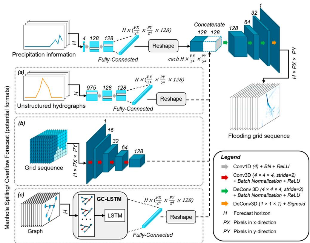
**Figure 7.** Baseline architecture with the different input paths for the considered formats of the overflow forecast. Baseline architecture with the input paths for the overflow forecast formatted as (a) unstructured hydrographs, (b) raster sequences, and (c) spatiotemporal graphs.
