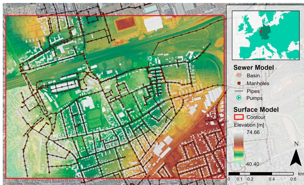
**Figure 2.** Illustration of the study area's sewer network and surface model (area outlined in red).
