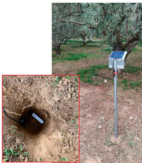
**Figure 6.** Installation of the soil moisture sensors as well as the IoT enabled device in the field.
