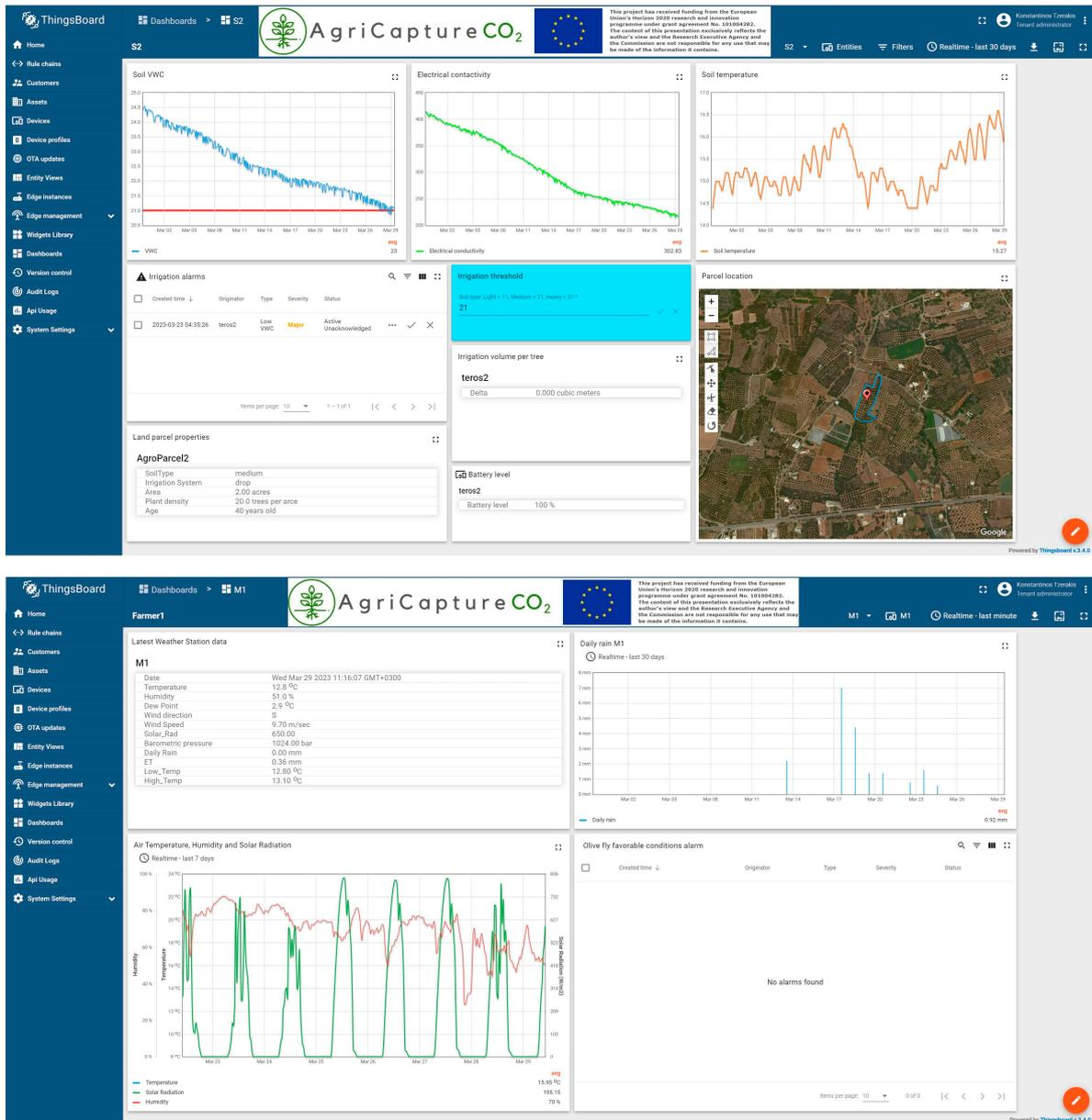
**Figure 7.** The public dashboard depicts soil moisture (VWC), electrical conductivity (ECa), soil temperature (°C) and irrigation needs/alerts (upper part). On the lower part of this figure, the basic weather data, as well as olive fruit fly alarms are displayed.
