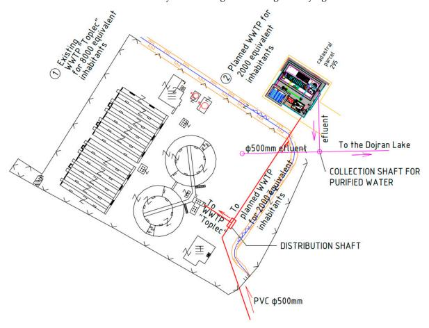
**Figure 1.** Combination of existing WWTP and new MBBR.
