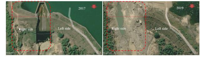
Figure 4. Collapsed spillway before and after the breach event (Google Earth images).
