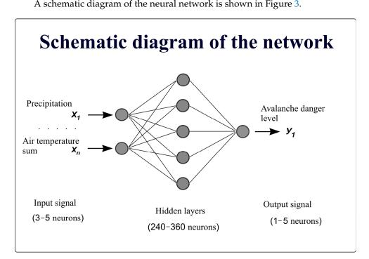
Figure 3. A schematic diagram of the artificial neural network.
