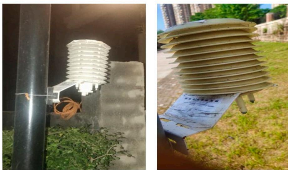
**Figure 3.** Small HOBO weather station.
