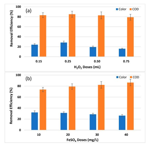
**Figure 6.** (a) Optimization of  $H_2O_2$  dose of raw pulp and paper wastewater for Fenton oxidation at different doses (0.15, 0.25, 0.50 and 0.75 mL). (b) Optimization of FeSO<sub>4</sub> dose of raw pulp and paper wastewater for Fenton oxidation at different doses (10, 20, 30 and 40 mg/L). Means values are presented with standard deviation.
