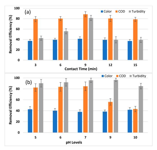
**Figure 3.** (a) Ozone treatment of raw wastewater and removal efficiencies (%) for color, COD and turbidity at varying contact times of 3, 6, 9, 12 and 15 min. (b) Ozone treatment of raw wastewater and removal efficiencies (%) for color, COD and turbidity at varying pH values (5, 6, 7, 9 and 10). Means values are presented in graphs with standard deviation.
