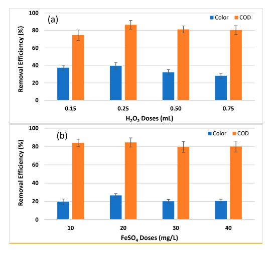
**Figure 7.** (a) Optimization of  $H_2O_2$  dose of treated pulp and paper wastewater for Fenton oxidation at different doses (0.15, 0.25, 0.50 and 0.75 mL) for biologically treated wastewater. (b) Optimization of FeSO<sub>4</sub> dose of treated pulp and paper wastewater for Fenton oxidation at different doses (10, 20, 30 and 40 mg/L) for biologically treated wastewater. Means values are presented with standard deviation.
