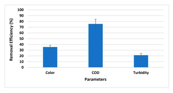
**Figure 8.** Fenton oxidation of chemically treated wastewater for removal of color, COD and turbidity. Means values are presented with standard deviation.
