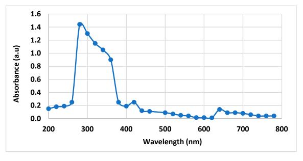
Figure 1. Absorption spectrum of raw wastewater from paper industry in the UV/Vis range.
