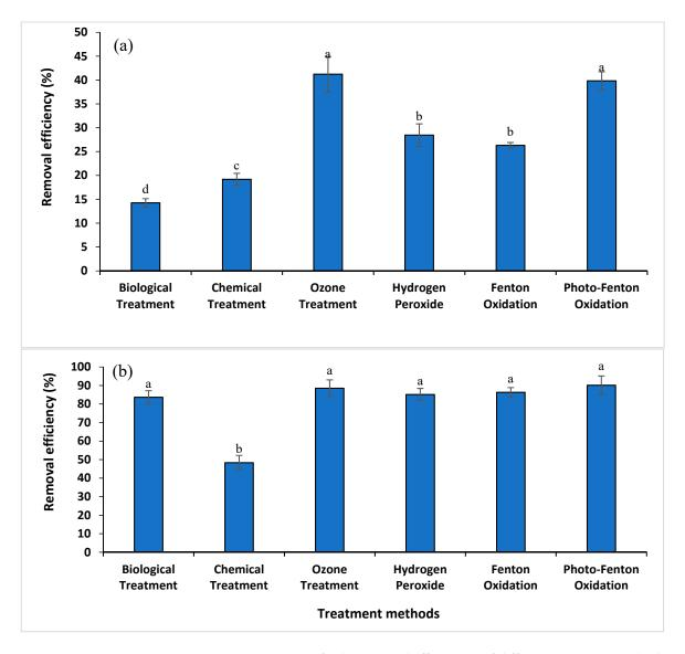
**Figure 10.** (a) Comparison of color removal efficiencies of different treatment methods applied to raw pulp and paper wastewater. (b) Comparison of COD removal efficiencies of different treatment methods when applied to raw pulp and paper wastewater. Mean values are presented with standard deviation. Different letters (a–d) show significant differences between treatments methods. Same letters (a, a, a) show that there is no significant difference between treatment methods.
