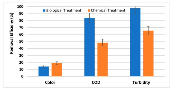
**Figure 2.** Removal efficiencies of biological treatment and chemical treatment of wastewater from pulp and paper industry for color, COD and turbidity. Mean values of percent removal of pollutant are presented with standard deviation.
