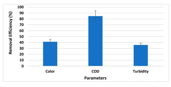
**Figure 5.** Ozone treatment of chemically treated wastewater and removal efficiencies (%) for color, COD and turbidity. Means values are presented in graphs with standard deviation.
