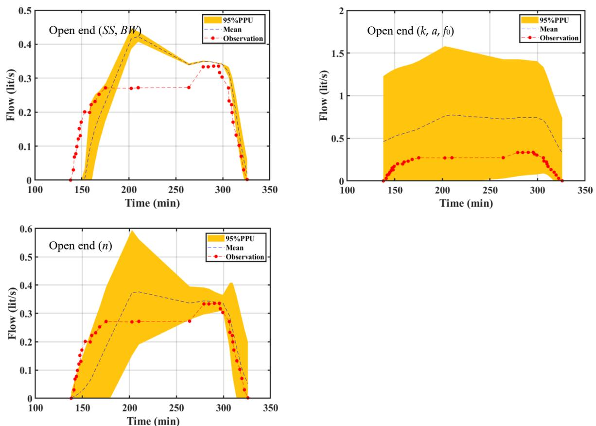
**Figure 3.** The uncertainty bounds of runoff hydrograph for open-ended furrow irrigation conditions and different parameters.
