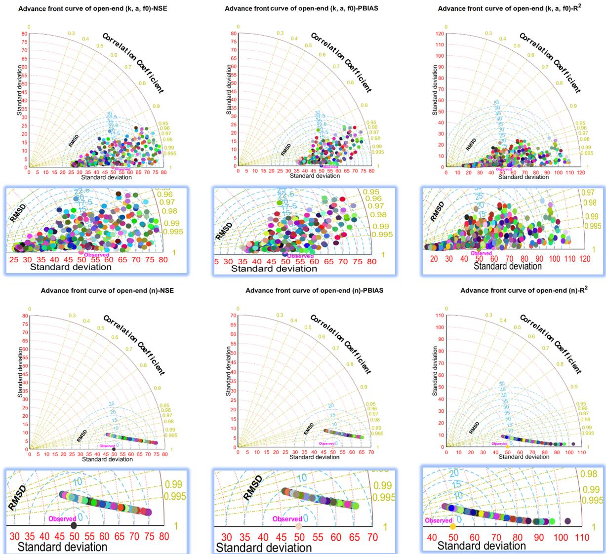
Figure 10. Taylor diagrams of WinSRFR advance front outputs for open-ended condition furrow irrigation after applying behavioral data.
