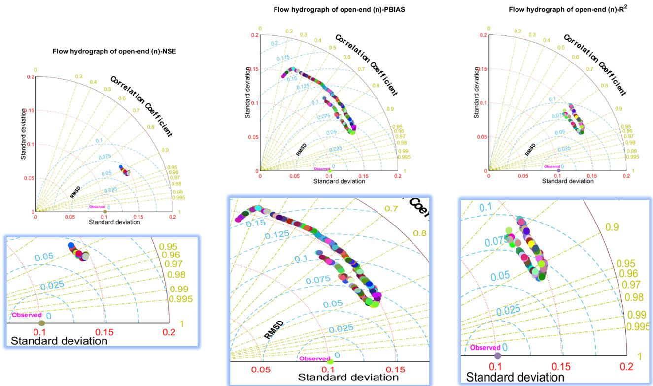
Figure 15. Taylor diagrams of WinSRFR runoff hydrograph outputs for open-ended condition furrow irrigation after applying behavioral data.
