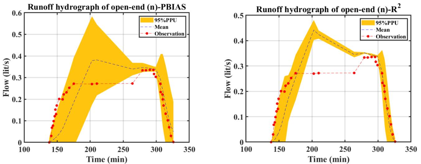
Figure 16. The uncertainty bounds of runoff hydrograph for different furrow irrigation conditions after removing non-behavioral data.
