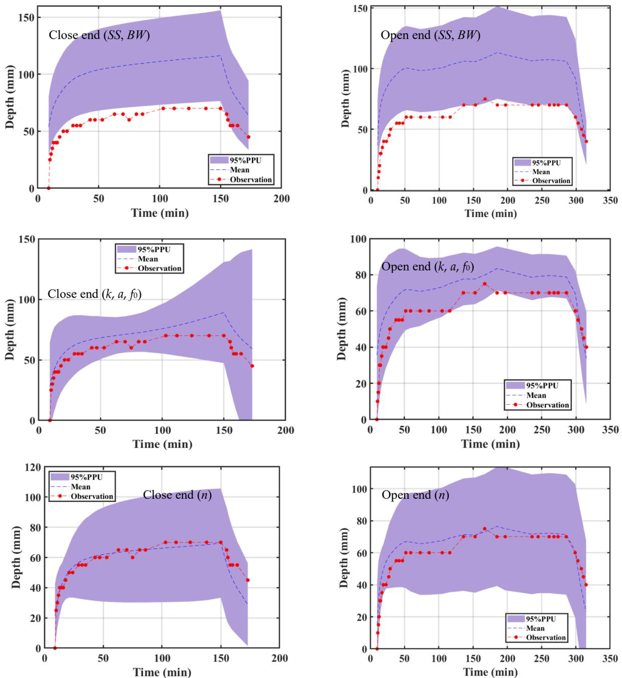
**Figure 2.** The uncertainty bounds of flow depth hydrograph for different furrow irrigation conditions and parameters.
