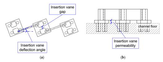
Figure 3. Schematic of the diversion vanes structural parameters. (a) Plan view; (b) side view.
