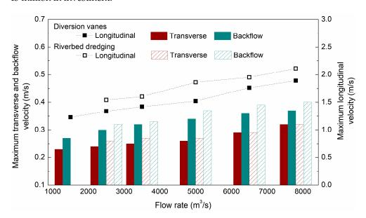
**Figure 13.** Comparison of navigable flow conditions between optimal riverbed-dredging and optimal diversion vanes schemes.
