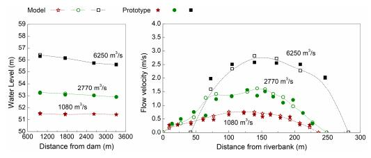
**Figure 7.** Comparison of water level and cross-section flow velocity between the prototype and the model.
