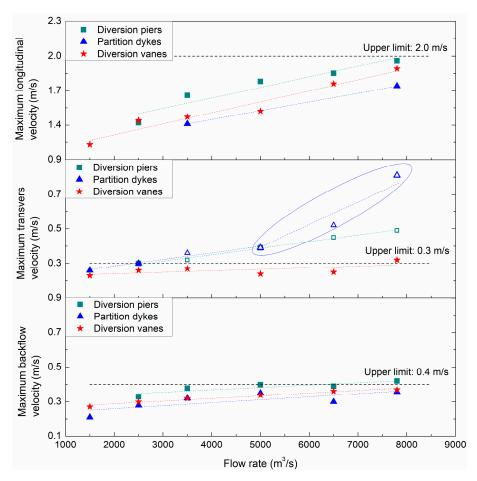
**Figure 11.** Distribution of extreme values of surface flow velocity at the entrance area of the approach channel of different diversion structures.
