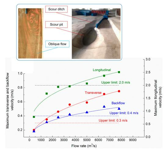
**Figure 9.** Surface velocity field and velocity extremums at the entrance area of the approach channel under current situations.
