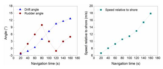
**Figure 16.** Change process of ship navigation parameters with navigation time at a typical flow rate  $(Q = 6500 \text{ m}^3/\text{s})$ .
