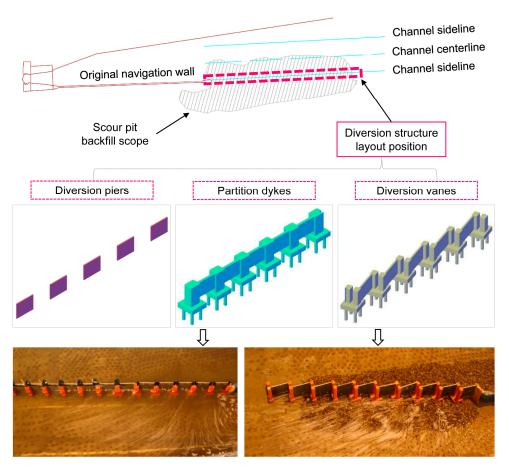
Figure 10. Schematic of optimal arrangement of different diversion structures.
