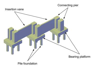
Figure 2. Schematic of the diversion vanes structure.
