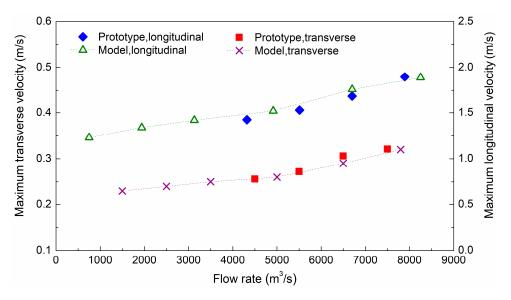
**Figure 15.** Comparison of extreme values of the surface flow velocity at the entrance area of the approach channel between the prototype and the model.
