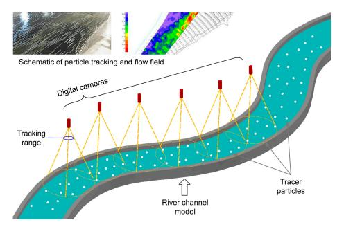
Figure 6. Schematic of the flow-field real-time measurement system (VDMS).
