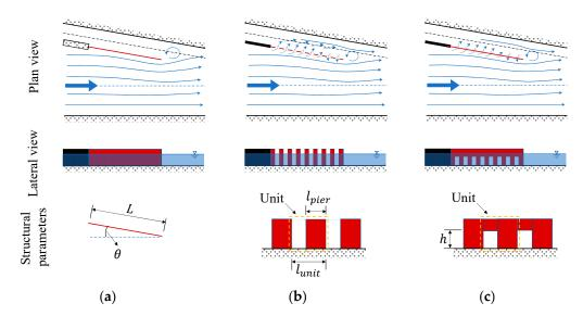
**Figure 1.** Schematic of three types of existing diversion structures. (a) Navigation wall, (b) diversion piers, and (c) partition dykes.
