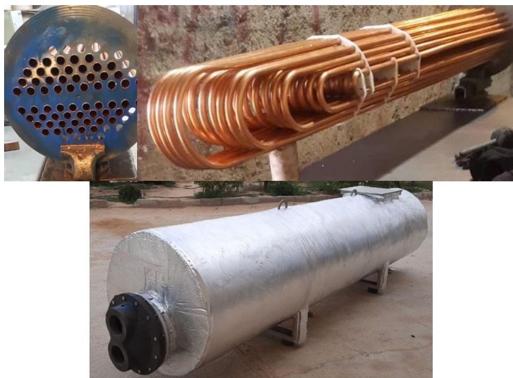
Figure 4. The thermal coil and the fabricated seawater tank.
