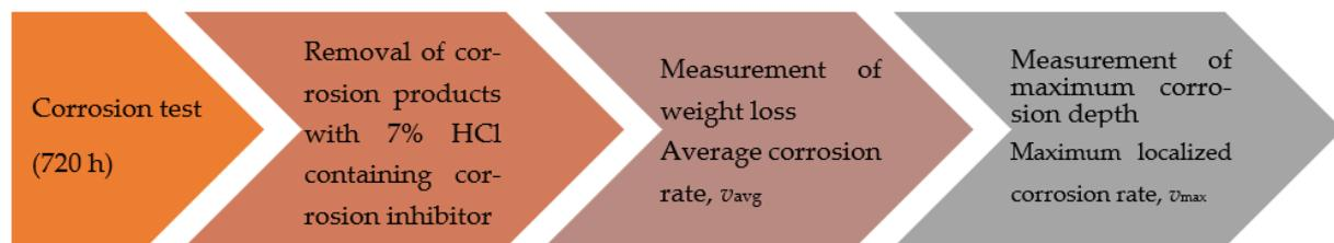
**Figure 3.** Process from surface treatment to measurement of corrosion.
