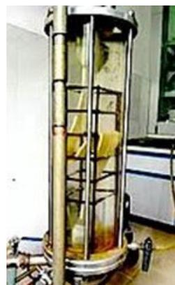
Figure 6. Water flow test model with typical bending patterns.
