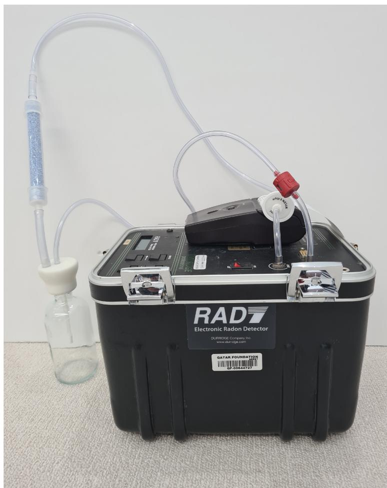
**Figure 2.** RAD7 with the RAD H<sub>2</sub>O accessory.
