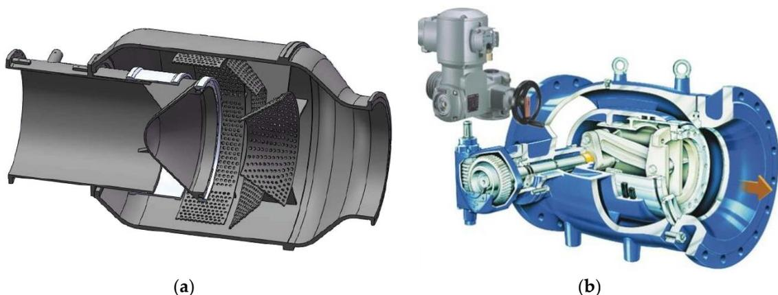
Figure 3. Test valves: (a) fixed cone valve; (b) plunger valve.
