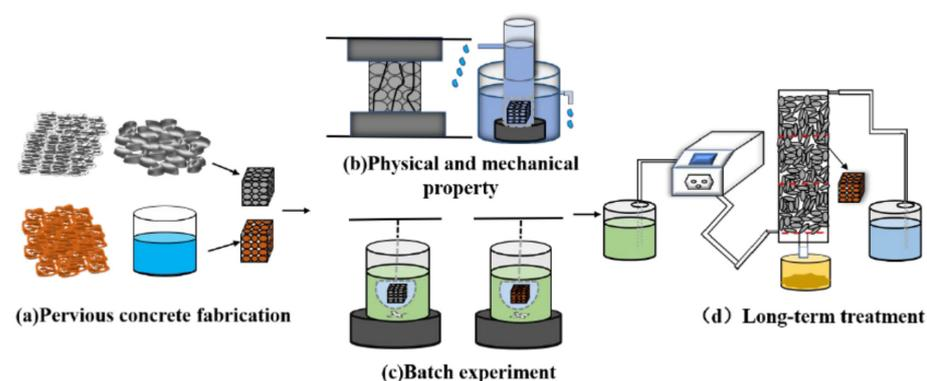
**Figure 10.** Experimental testing scheme for potential application of permeable materials in pollutant removal: (a) preparation of the monolith sample; (b) physical and mechanical characterizations; (c) static removal test; (d) dynamic removal test (copyrighted from [30]).
