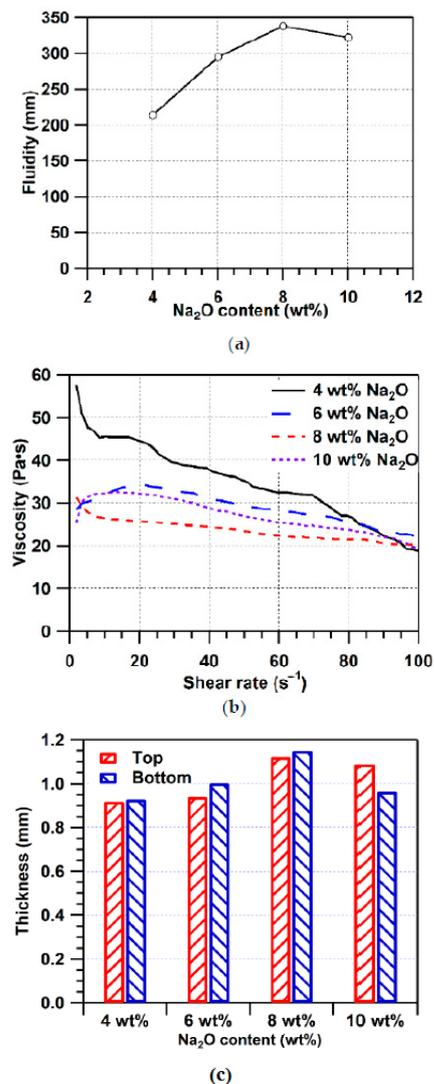
**Figure 8.** Effect of the variation of the mix design on the paste's properties in innovative permeable concrete: (a) fluidity; (b) viscosity and shear stress; (c) coat thickness (copyrighted from [131]).
