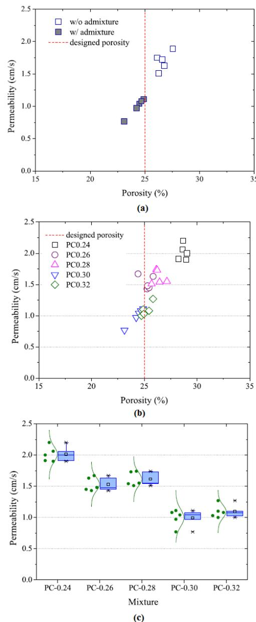
**Figure 9.** Effects of the mix design on the hydraulic properties of the hardened permeable concrete of different water to cement ratio PC-X (X = 0.24; 0.26; 0.28; 0.3; 0.32): (a) effect of the incorporation of the admixture; (b) effect of the w/c ratio; (c) statistical distribution of the permeability at different w/c ratios (copyrighted from [123]).
