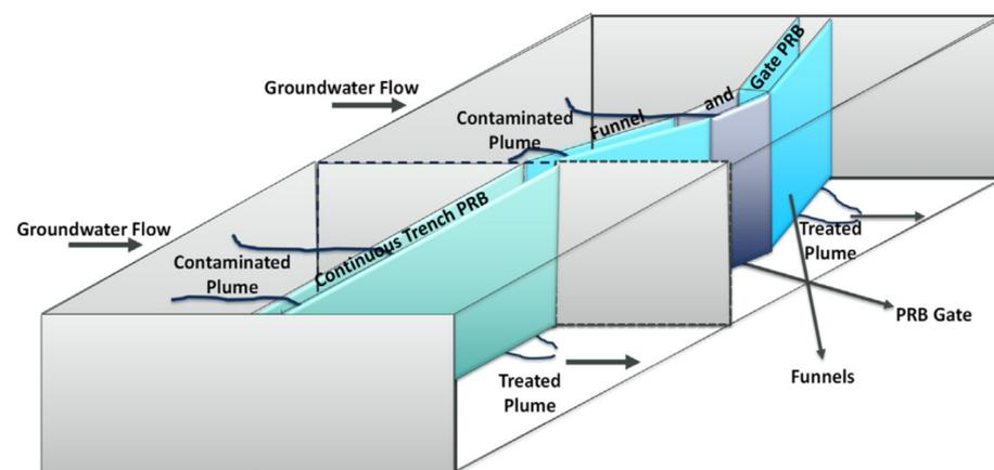
Figure 11. Configuration of the PRB designs: (copyrighted from [161]).
