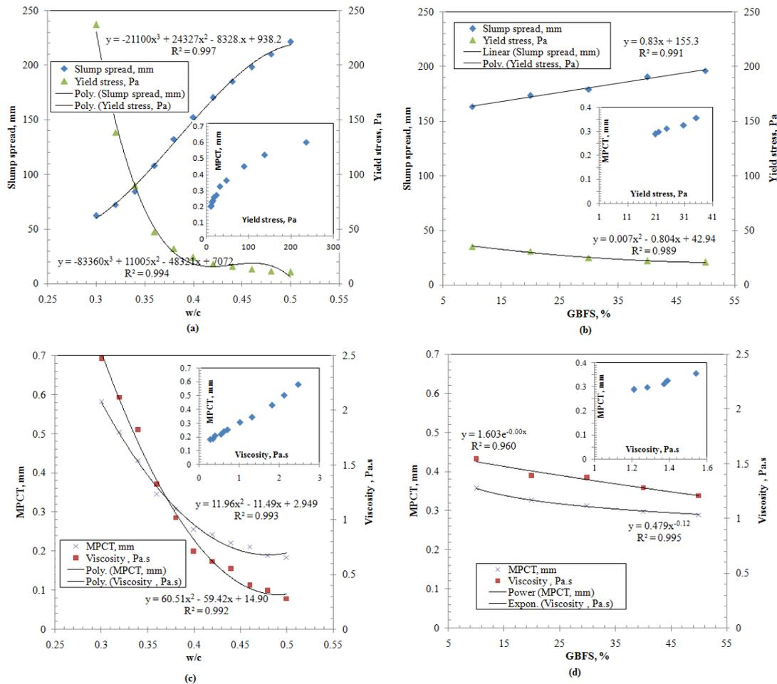
**Figure 7.** Effect of the mix design variation on the paste properties in conventional permeable concrete: (a,c) effect of the w/c ratio variation; (b,d) effect of the GBFS in cooperation (source data were extracted from [124]).
