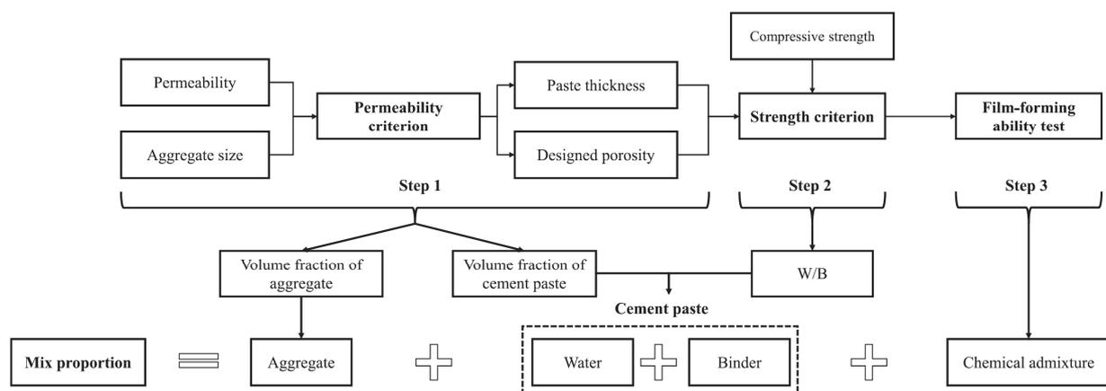
**Figure 4.** Proposed procedure to optimize the mix design of permeable concrete based on the permeability and compressive strength (copyrighted from [113]).
