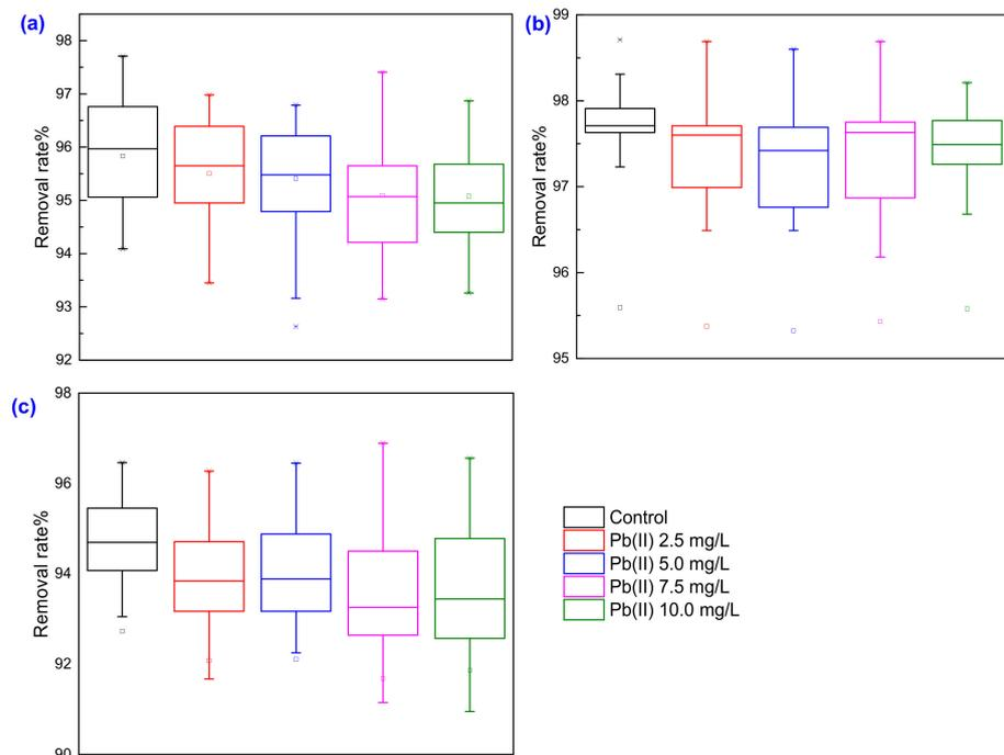
**Figure 7.** Removal profiles of COD (a), ammonia-N (b) and phosphate-P (c) across ninety days of operation. The symbols of ‘□’ and ‘\*’ in the figures stand for average value and outside point, respectively.
