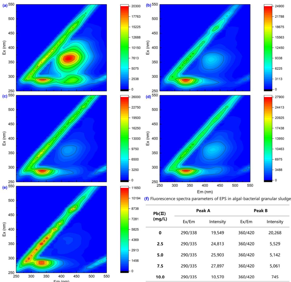
**Figure 4.** 3D-EEM spectra of EPS from algal-bacterial granular sludge after 90 day-culture in the presence of Pb(II) (a)–0; (b)–2.5 mg/L; (c)–5.0 mg/L; (d)–7.5 mg/L; (e)–10.0 mg/L) and the fluorescence spectra parameters (f).
