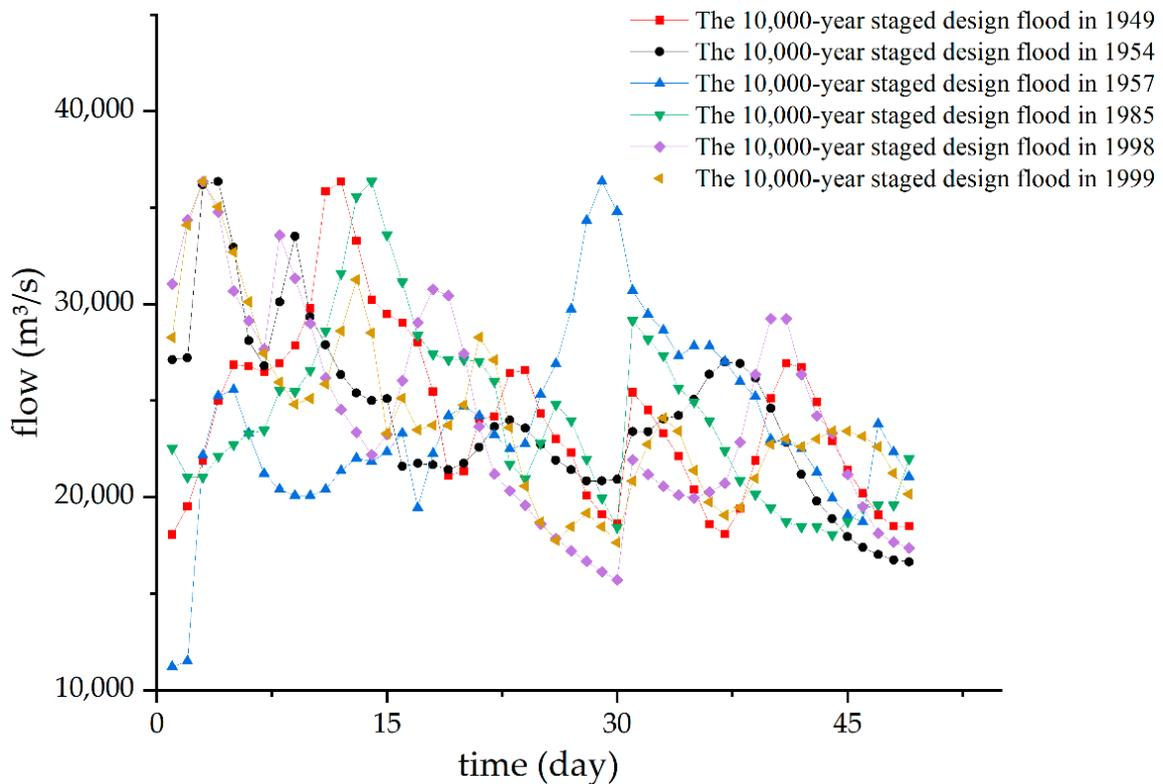
Figure 4. The 0.01% staged design floods for the Baihetan Reservoir.
