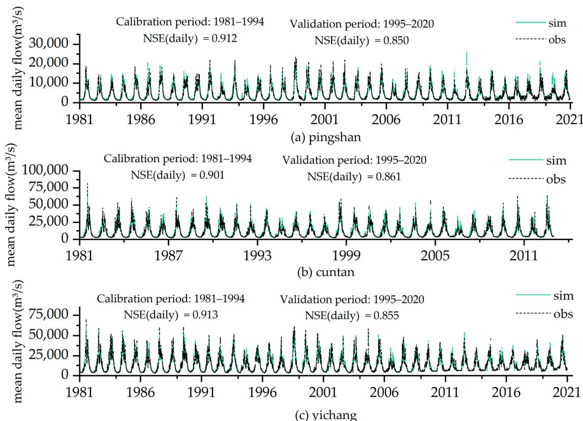
**Figure 2.** The simulated and observed daily streamflow at (a) Pingshan, (b) Cuntan, and (c) Yichang.
