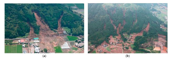
**Figure 3.** The landslides caused by heavy rain. **(a)** Shallow landslide that occurred in Ichinomiya Town, Aso City, Kumamoto Prefecture. **(b)** Debris flow that occurred in Kitanosaka-nashi, Ichinomiya Town, Aso City, Kumamoto Prefecture. The photos were provided by Asia Air Survey Co., Ltd.
