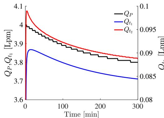
**Figure 2.** Transient pumping flow rate ( $Q_p$ ) defined from the exponential model provided in (A18) with  $Q_{t_1} = 4$  and  $Q_{t_2} = 3.8$  Lpm at times  $t_1 = 0$  and  $t_2 = 300$  min with the fitting coefficient  $b$  set to  $10^5$ .  $Q_p$  is the pumping flow rate considered in *Config3* of Section 3.2 and in all the experiments in Section 3.3.  $Q_{t_1}$  and  $Q_{t_2}$  correspond to the aquifer flow rates of the reference experiments considered in Section 3.3.
