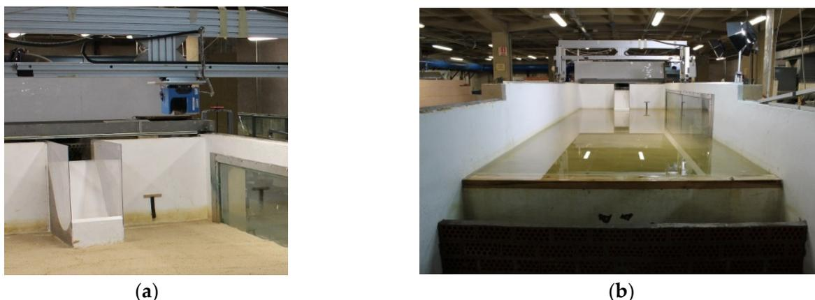
**Figure 5.** (a) Testing area with spillway. Case:  $R = 0.4$  m;  $\alpha = 45^\circ$ ; (b) view of the testing channel from downstream with a water cushion.
