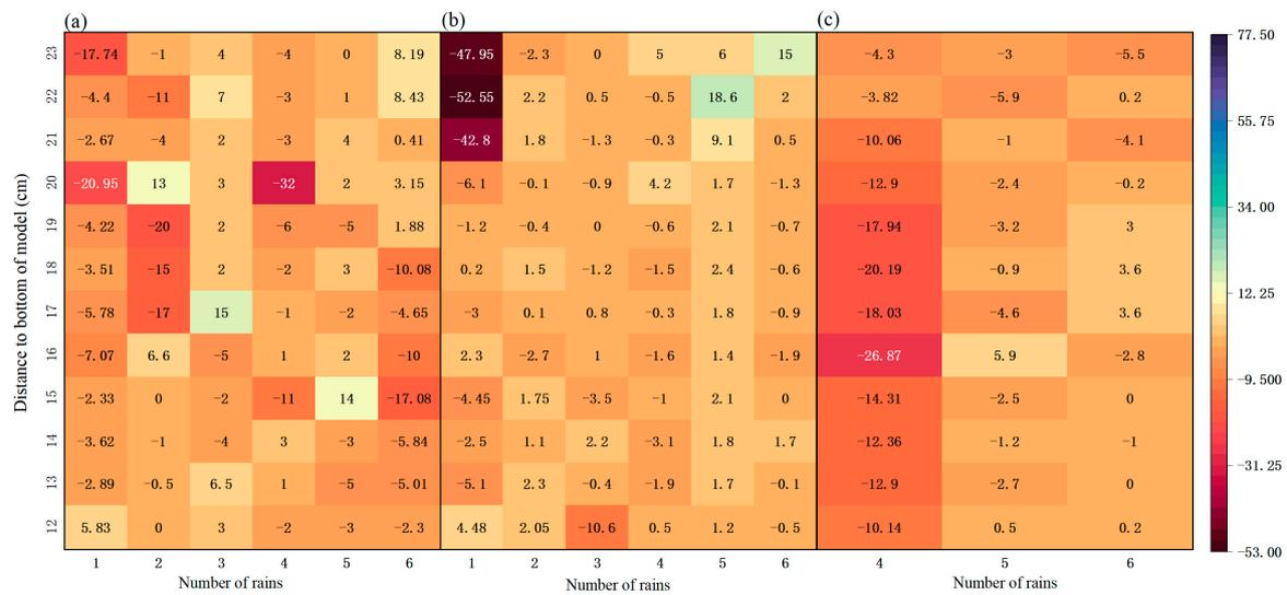
**Figure 3.** Changes in relative depth after simulated rainfall in different measures. (a) LT measure; (b) NDT measure; (c) DT measure (Note: since the first three rainfalls in the DT measure, the water flow is all discharged from the drainage pipe and does not pass through the slope, so only the relative depth changes in the last three rainfalls are measured).
