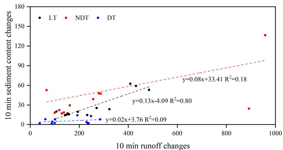
**Figure 6.** Relationship between 10 min runoff and 10 min sediment content changes in different measure types under different rainfall.
