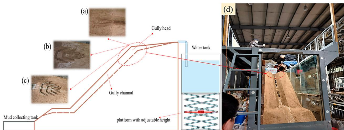
**Figure 1.** Schematic diagram and model diagram of slope scour model test. (a) LT measure; (b) NDT measure; (c) DT measure; (d) Scour model diagram.
