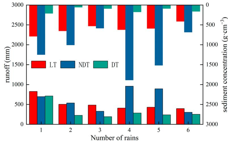
**Figure 4.** Runoff and sediment concentration with three measures during simulated rainfall. (Note: the bar graph above the figure represents sediment concentration, while the bar graph below represents runoff.)
