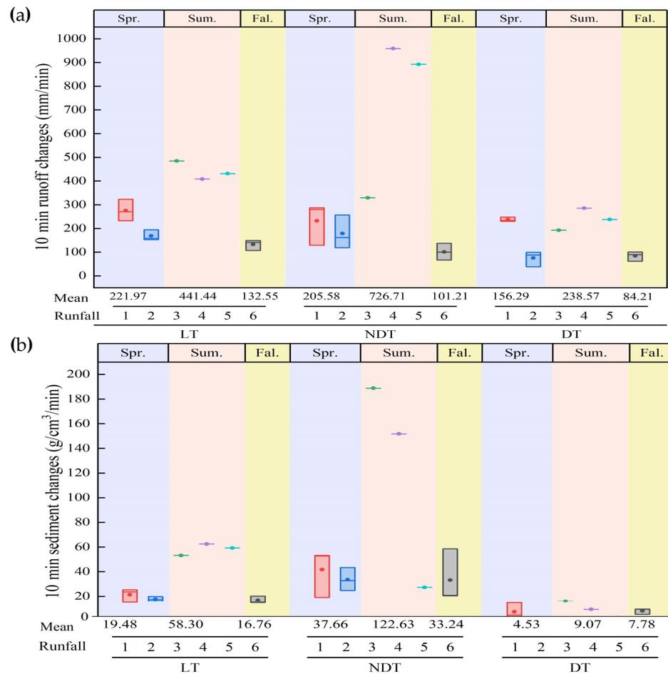
**Figure 5.** Ten min runoff changes and sediment content changes on the loess slope with different measures during simulated rainfall. (a) Ten min runoff changes; (b) Ten min sediment changes. (Note: Since the rainfall duration in both spring and fall is 30 min, the dots in the box plot represent the mean values of the changes in runoff and sediment concentration averaged over three 10 min intervals. The “mean” label below indicates the specific average values.)
