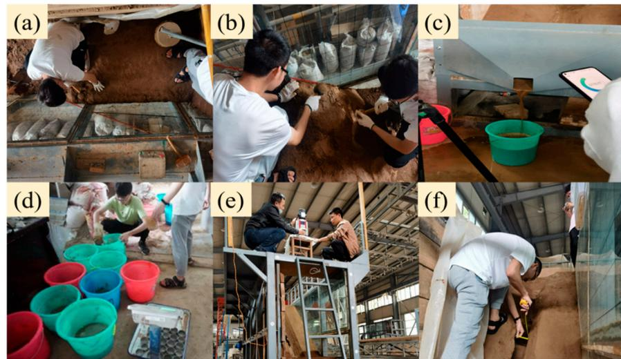
**Figure 2.** Schematic diagram of model design and monitoring. (a) Compacting soil layer; (b) Slope cutting along predetermined slope line; (c) Recording bucket replacement time; (d) Sampling and weighing; (e) Taking photos of the channel; (f) Measuring channel changes.
