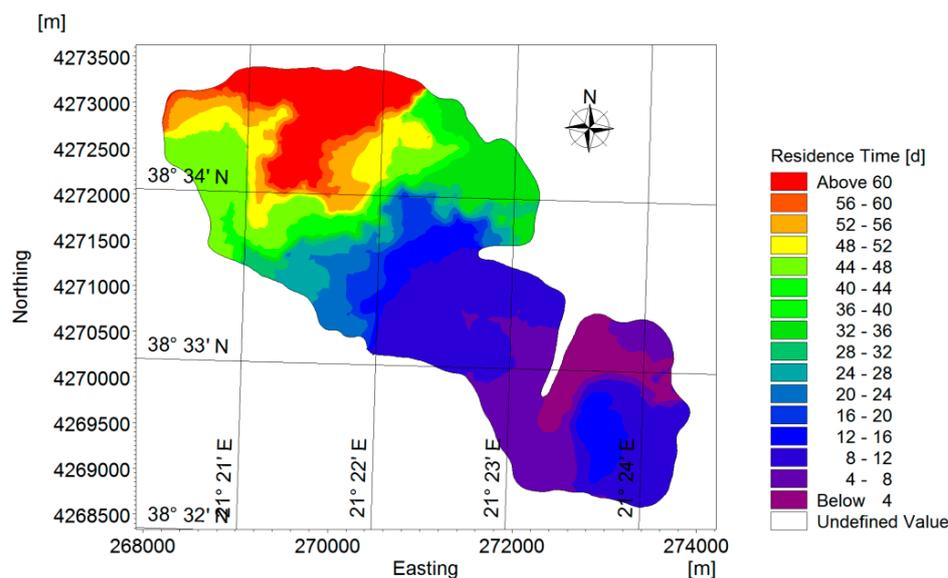
**Figure 10.** Distribution of residence time in the surface waters of Lysimachia Lake. Results are given for a 60-day simulation.
