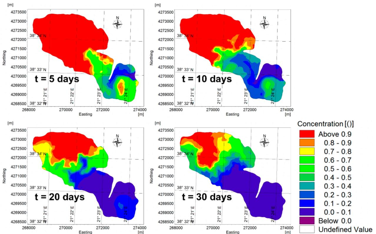
**Figure 9.** Distribution of the numerical tracer concentration inside Lysimachia Lake after 5, 10, 20 and 30 days.
