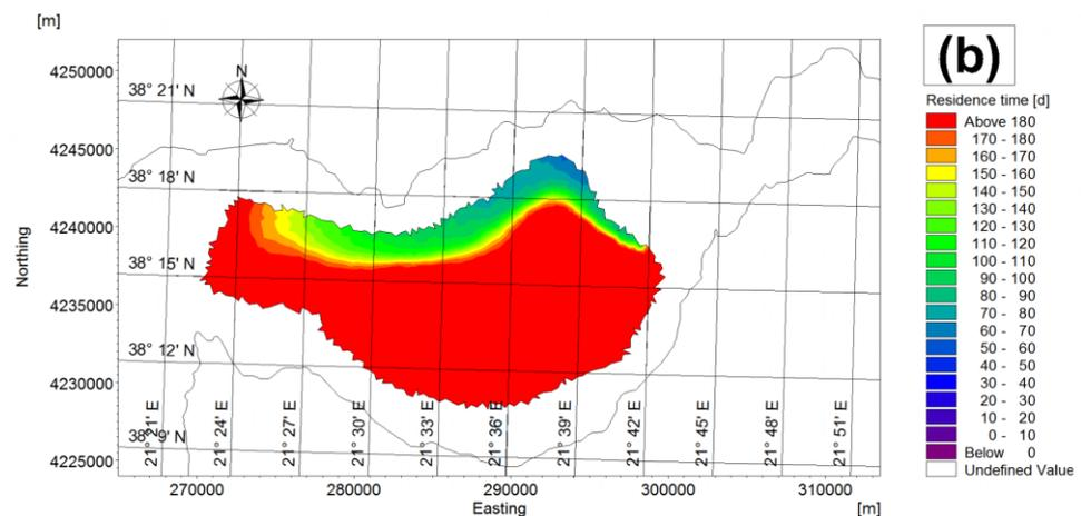
**Figure 7.** Distribution of residence time (a) in the surface waters of the Gulf of Patras basin and (b) in the deeper and bottom waters of the Gulf (>60 m), enclosed between the two sills. Results are given for a 6-month simulation.
