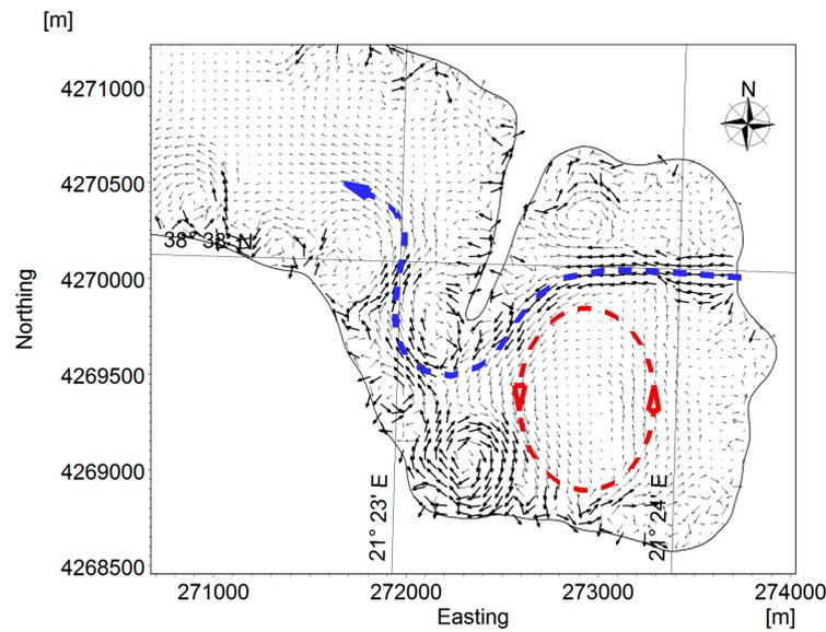
**Figure 8.** Main circulation pattern of the flow field in the eastern part of the Lake after steady state is reached.
