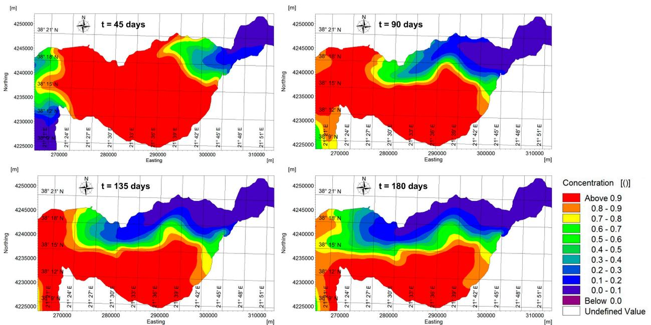
Figure 6. Comparison of the evolution of the concentration field of the numerical tracer in the Gulf of Patras at 45, 90, 135 and 180 days from the start of the simulation.
