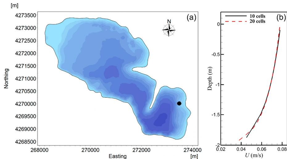
**Figure 3.** (a) The position of the point in the eastern part of the Lake (marked with black dot), where the U-velocity profile was taken, and (b) U-velocity profile for the two different discretizations used for the mesh sensitivity analysis.
