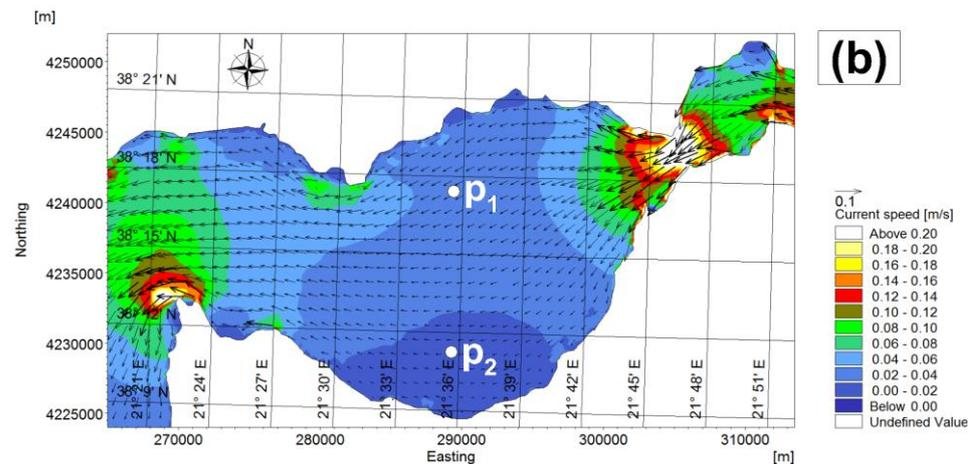
**Figure 4.** Surface currents in the Gulf of Patras under windless conditions in phase of (a) flood and (b) ebb tide.
