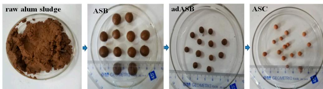
**Figure 1.** Each production stage of ASC and its apparent change.
