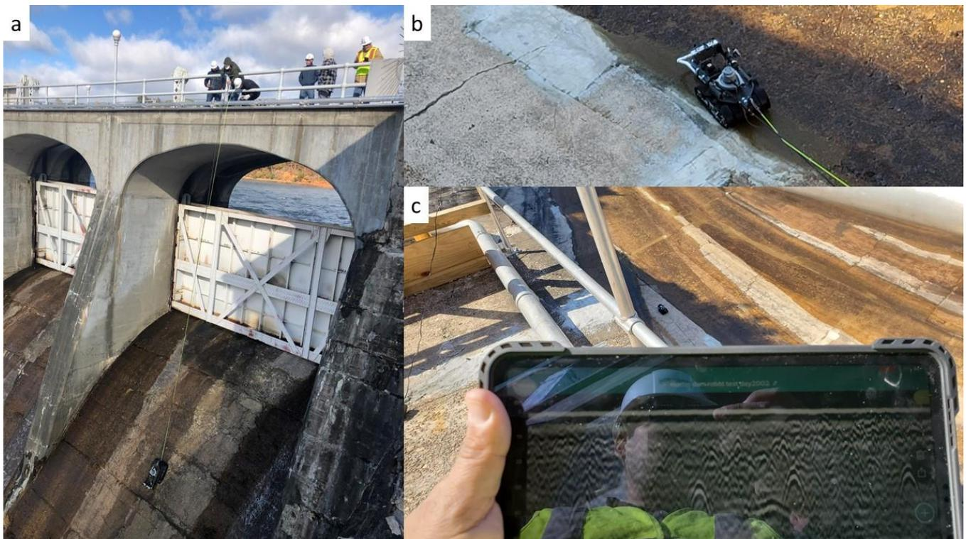
Figure 4. Photographs showing (a) crawler with GPR being lowered onto spillway, (b) crawler with GPR collecting data across repaired concrete surface, and (c) data collection with iPad from top of dam with crawler with GPR in background.
