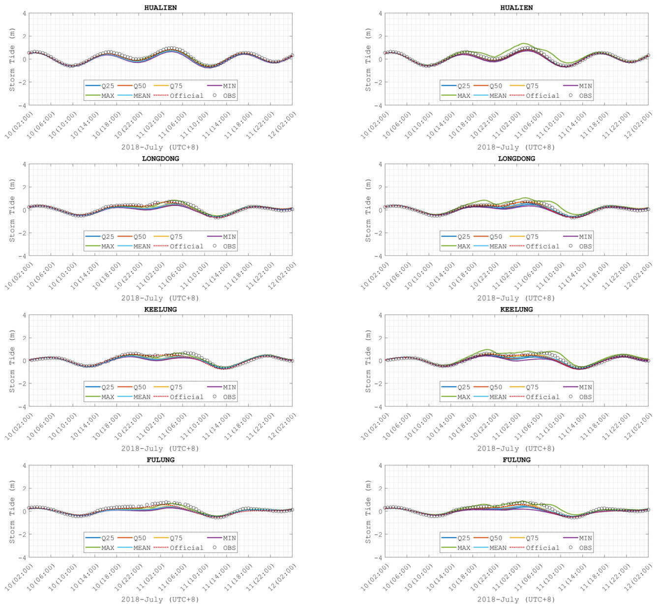
Figure 10. Time series of ensemble statistical results of storm tide. Black circles are observation. The left shows the statistic results from WEPS, and the right is from EDF, including quartiles, minimum, maximum, and mean of ensembles.
