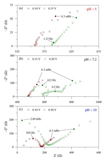
**Figure 4.** Electrochemical impedance spectroscopy spectra for the  $0.001 \, \mathrm{M} \, \mathrm{H_x PO_4}^{3-x}$  solution at **(a)** pH 5, **(b)** pH 7, and **(c)** pH 10. The impedances were obtained at bias potentials comprehending  $i < i_{lim,1}$  (red) and  $i = i_{lim,1}$  (green) region of the polarization curve. Solid points refer to characteristic frequencies.
