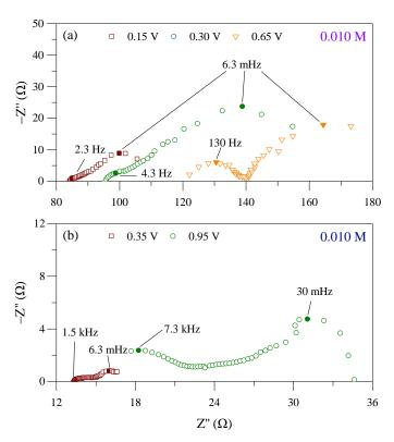
**Figure 6.** Electrochemical impedance spectroscopy spectra for the (a) 0.01 M and (b) 0.1 M  $H_xPO_4^{3-x}$  solution at pH 7.2. The impedances were obtained at bias potentials comprehending the  $i < i_{lim,1}$  (red),  $i = i_{lim,1}$  (green), and  $i_{lim,1} < i < i_{lim,2}$  (orange, when applicable) region of the polarization curve. Solid points refer to characteristic frequencies.
