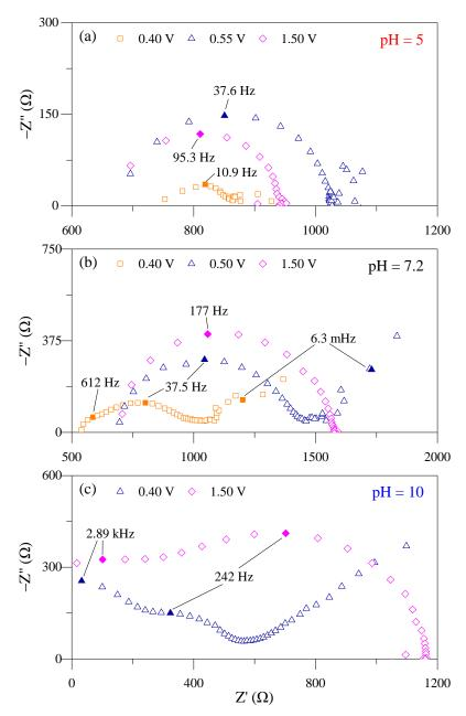
**Figure 5.** Electrochemical impedance spectroscopy spectra for the 0.001 M  $H_xPO_4^{3-x}$  solution at (a) pH 5, (b) pH 7 and (c) pH 10. The impedances were obtained at bias potentials corresponding to the  $i_{lim,1} < i < i_{lim,2}$  (orange, when applicable),  $i = i_{lim,2}$  (blue) and  $i > i_{lim,2}$  (pink) region of the polarization curve. Solid points refer to characteristic frequencies.
