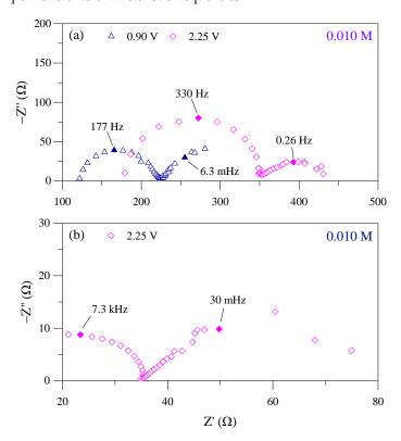
**Figure 7.** Electrochemical impedance spectroscopy spectra obtained at bias potentials corresponding the  $i = i_{lim,2}$  (blue) and  $i > i_{lim,2}$  (pink) for the (a) 0.01 M and (b) 0.1 M  $H_xPO_4^{3-x}$  solution at pH 7.2. For the 0.1 M solution, only  $i_{lim,1}$  was reported. Solid points refer to characteristic frequencies.
