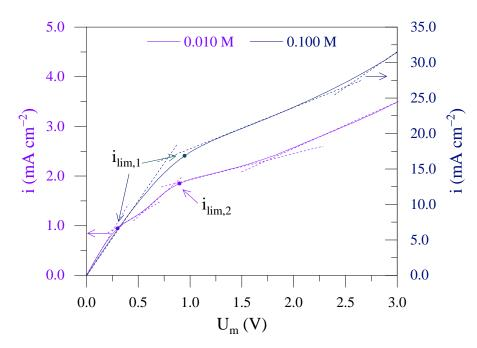
**Figure 3.** Polarization curves for the IONSEP-HC-A membrane in contact with a solution with 0.010 M and 0.100 M of  $H_xPO_4^{3-x}$  at pH 7.2. Dotted lines represent the delimitation of polarization curve regions.
