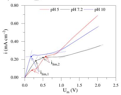
**Figure 2.** Polarization curves for the IONSEP-HC-A membrane in contact with a solution with 0.001 M of  $H_xPO_4^{3-x}$  at pH 5 (red line), 7.2 (black line), and 10 (blue line). Dotted lines represent the delimitation of polarization curve regions.
