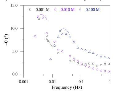
**Figure 8.** Bode plot of the phase angle versus the frequency for the three  $H_xPO_4^{3-x}$  concentration conditions at pH 7.2. The bias potential applied comprehends the last plateau region of each experimental condition.
