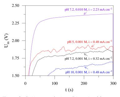
**Figure 9.** Overlimiting current density condition section of chronopotentiometric curves for different experimental conditions.
