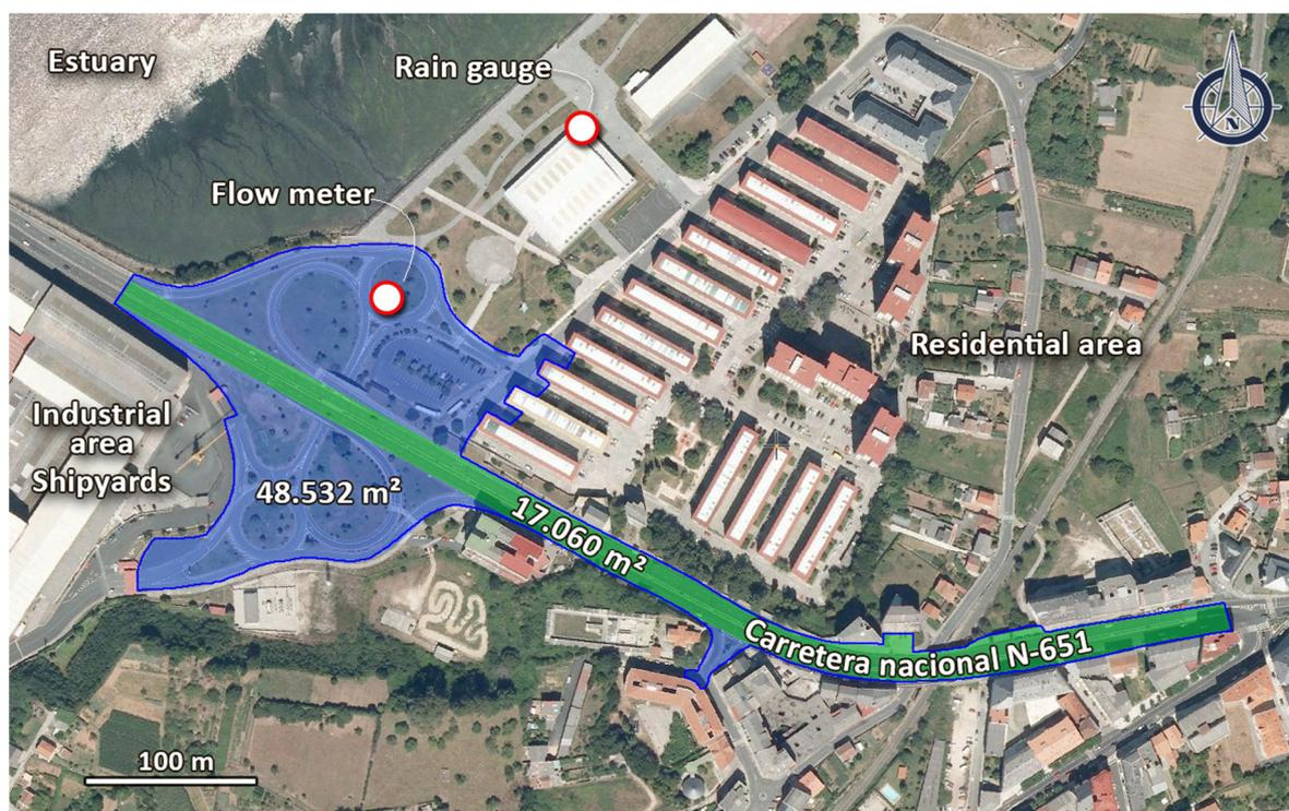
**Figure 1.** Road surface and adjacent areas of the study basin in Fene (A Coruña, Spain). Study basin marked in blue and green.
