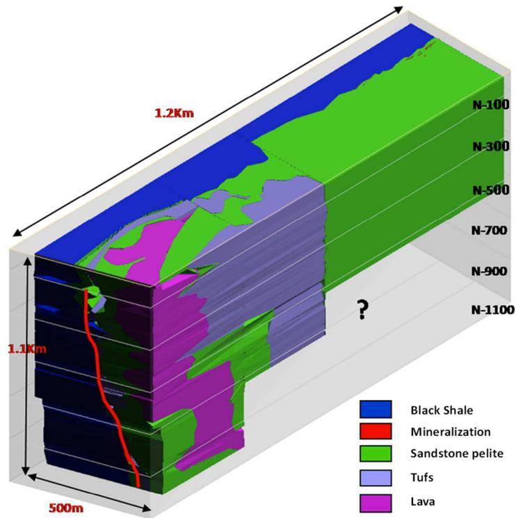
Figure 2. 3D geological block diagram of the Draa Sfar deposit [22].
