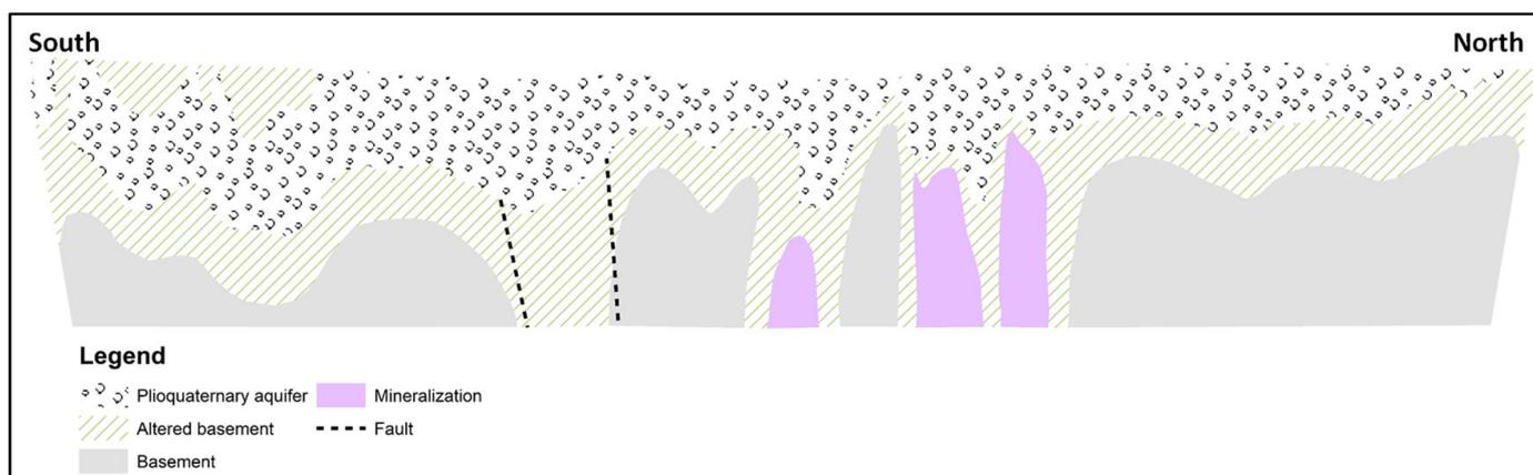
**Figure 3.** Geohydrological conceptual model of the study area.
