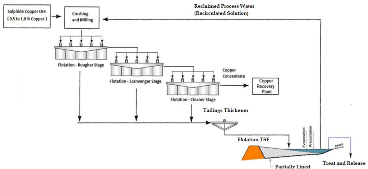
Figure 5. Typical sulphide copper ore flowsheet process—copper mine tailings management [4].
