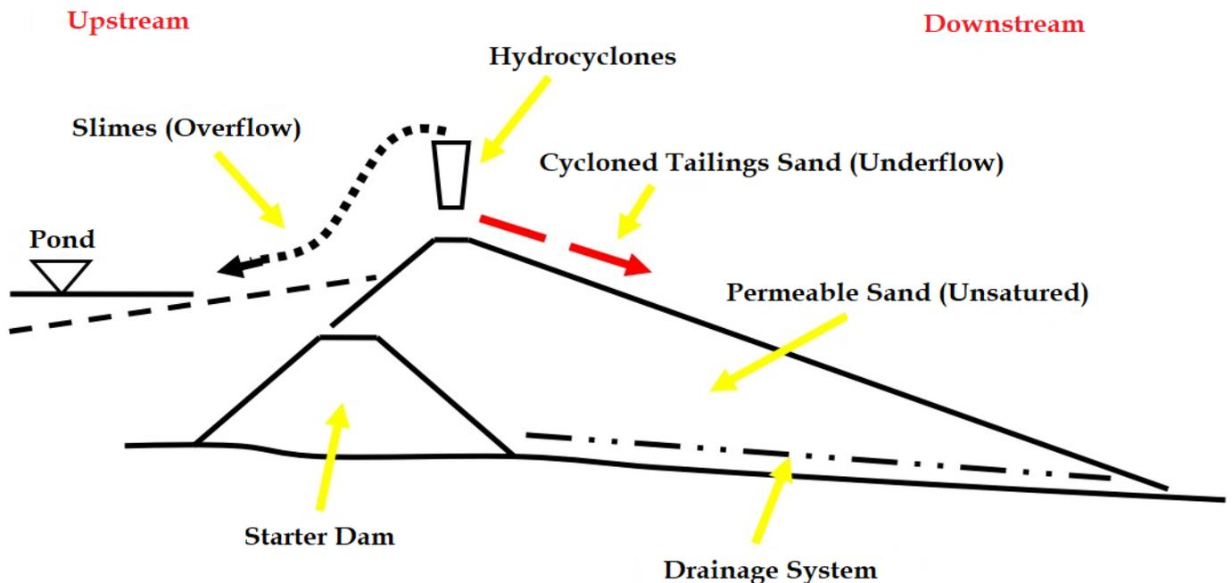
Figure 18. Schematic view of cycloned tailings sand dam construction.
