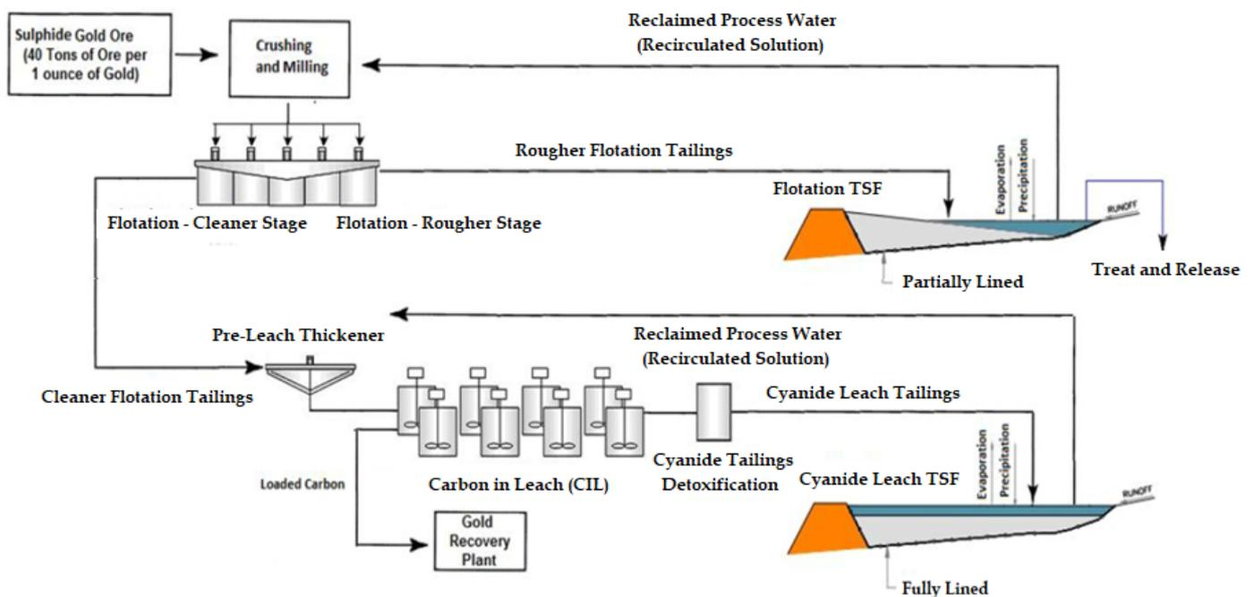
**Figure 3.** Typical sulphide gold ore flowsheet process—gold mine tailings management [4].
