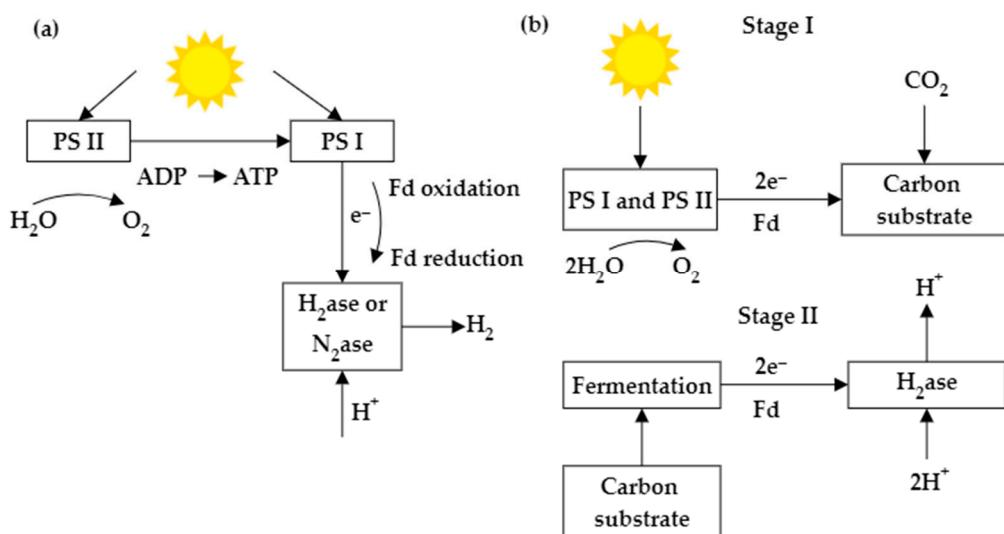
**Figure 1.** Schematic diagram of bioH<sub>2</sub> production through (a) direct biophotolysis and (b) indirect biophotolysis.
