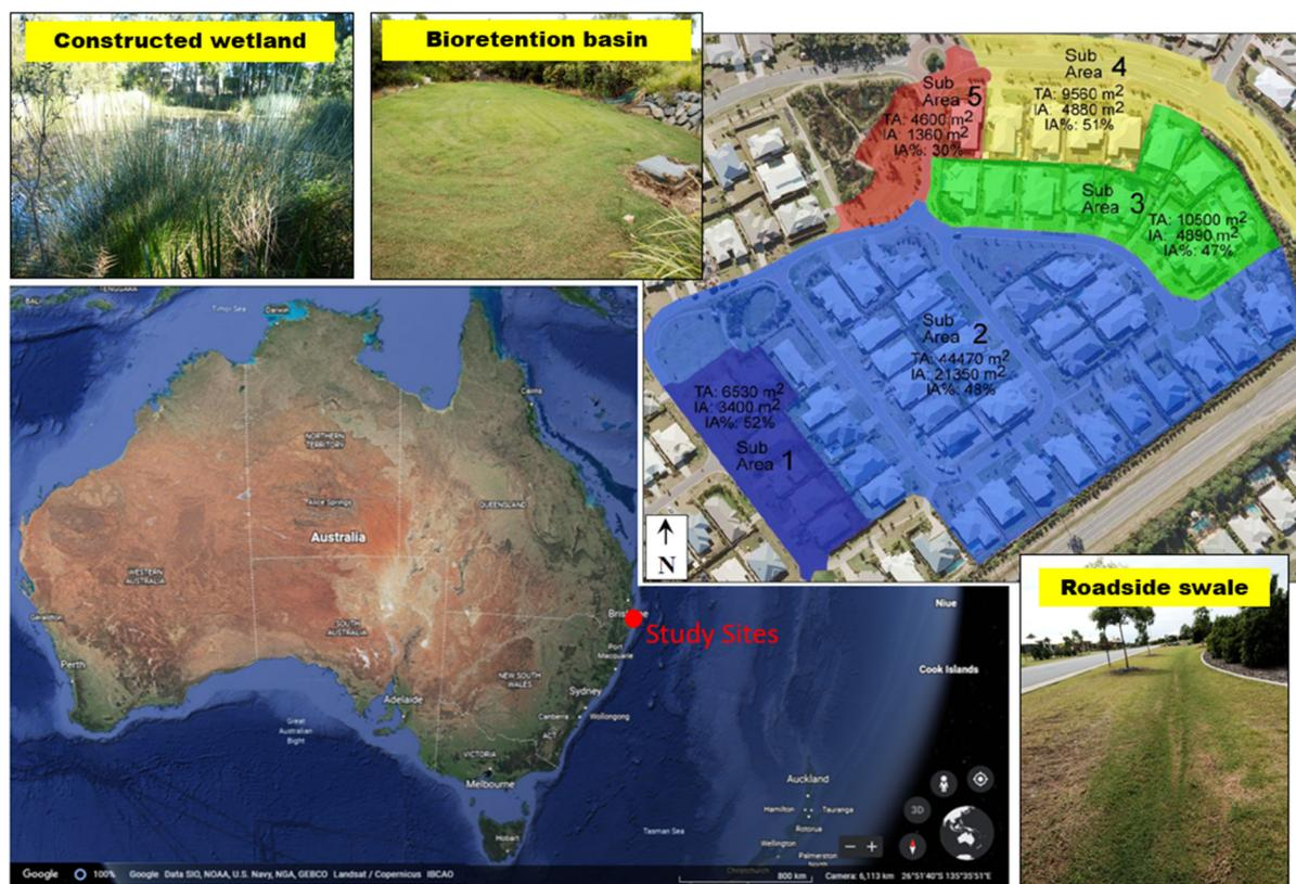
**Figure 1.** Study site. TA: total area; IA: impervious surface area; IA%: impervious surface percentage. Stormwater runoff from sub-area 1 primarily contributes to B. After passing through B, the stormwater enters the constructed wetland. Stormwater runoff from sub-area 2 and sub-area 3 directly flows to W. Sub-area 4 distributes flow to roadside swales, while sub-area 5 is the bypass of W, which does not receive treatment from any of the WSUDs.
