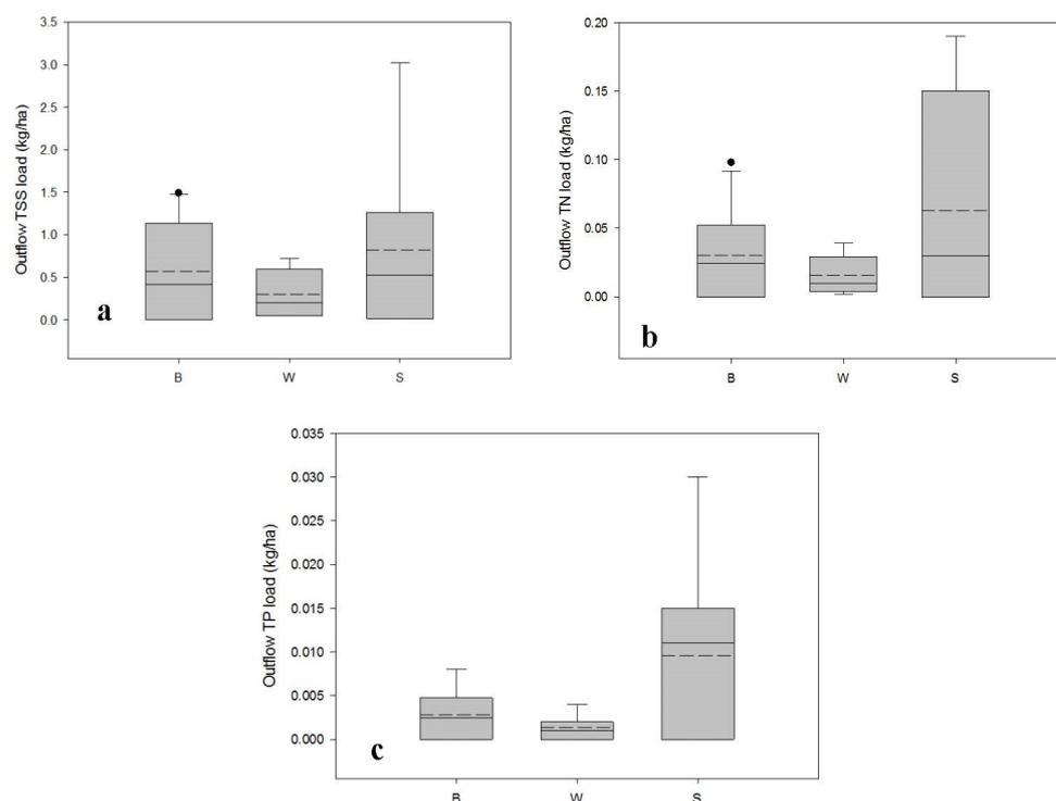
**Figure 4.** Outflow pollutant loads of WSUDs, (a) TSS; (b) TN; (c) TP. B = bioretention basin; W = constructed wetland; S = roadside swale.
