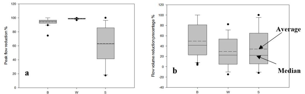
**Figure 2.** Hydraulic performance of WSUDs, (a) peak flow reduction; (b) flow volume reduction. B = bioretention basin; W = constructed wetland; S = roadside swale.
