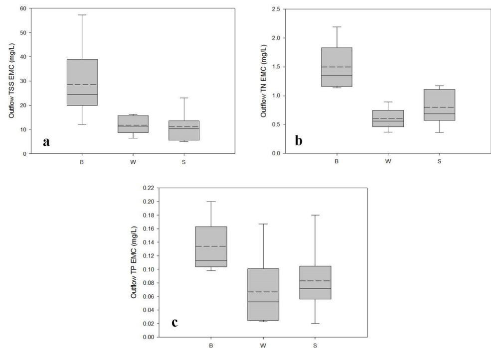
**Figure 3.** Outflow pollutant EMCs of WSUDs, (a) TSS; (b) TN; (c) TP. B = bioretention basin; W = constructed wetland; S = roadside swale.
