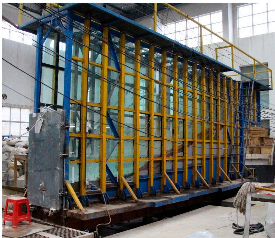
Figure 4. Landslide model test system.
